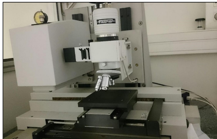
Figure 5: Micro-indenter Fischerscope H100C XYp.
