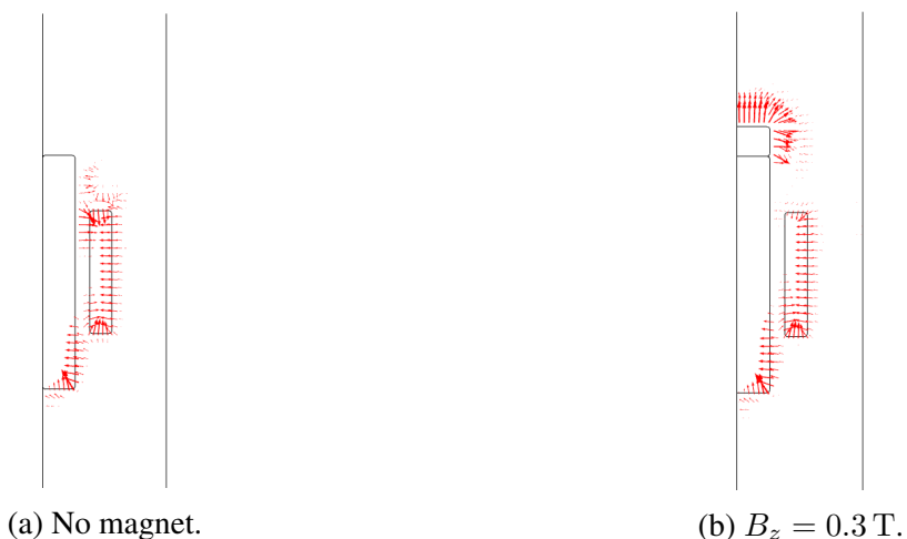
Figure 3.49: Helmholtz force distributions in the two presented cases.
