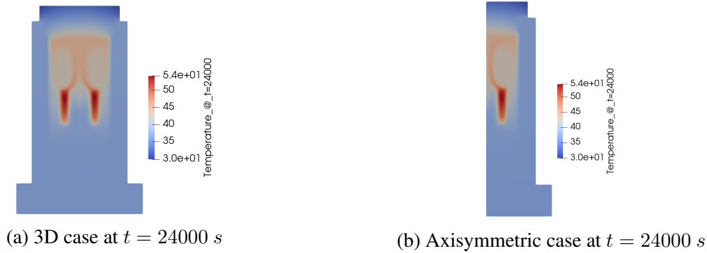
Figure 4.3: Temperature field (in ^{\circ}\text{C} ) when the magnetic force is inactive. The symmetry axis ( Oz ) is on the left for the axisymmetric model (panel b).
