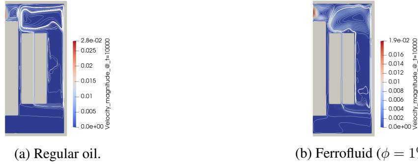
Figure 4.13: Distribution of the velocity magnitude (in \text{m s}^{-1} ) at t = 10\,000\text{ s} .
