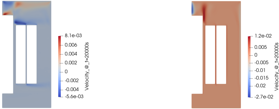
(a) Radial component of the velocity field u_r , symmetry axis at the left. (b) Axial component of the velocity field u_z , symmetry axis at the left.
