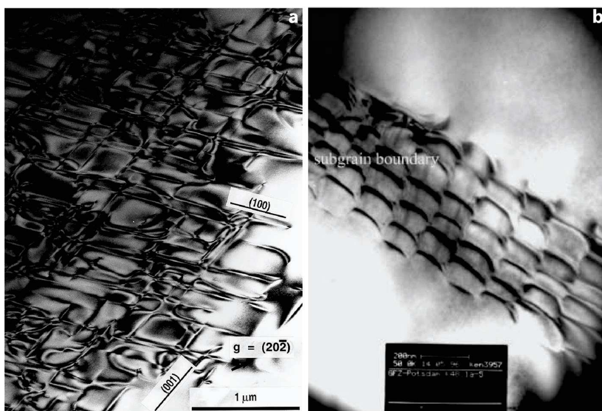
Figure 1.21 - Transmission Electron Microscopy (TEM) microphotographs of dislocations. (a) Two set of dislocations, parallel to (001) and (100) crystallographic planes, forming numerous rectangular loops in plagioclase (Kruse & Stünitz, 1999). (b) Subgrain boundary indicative of climb in amphibole (Kenkmann & Dresen, 2002).
