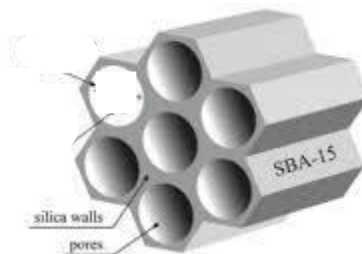
Figure I.21: Hexagonal porous structure of SBA-15 [183]
