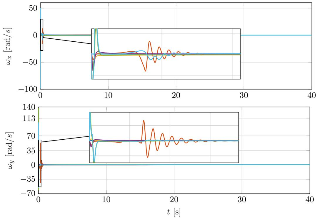
Figure 6.14: Angular rates of the UAVs in the directed scenario.
