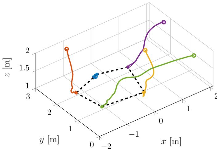
Figure 6.18: Paths followed by the DJI Tello drones up to the desired pentagonal formation.
