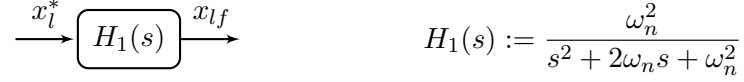
Figure 5.2: Command filter used for implementation. The dirty derivative of x_l^* may be obtained using \dot{x}_{lf} := sH_1(s)x_l^* which is equivalent to \dot{x}_{lf} = H_1(s)\dot{x}_l^* .
