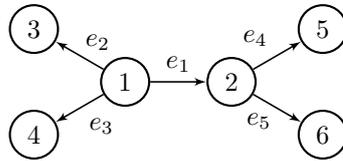
Figure 6.9: Directed-spanning-tree graph at the initial time.
