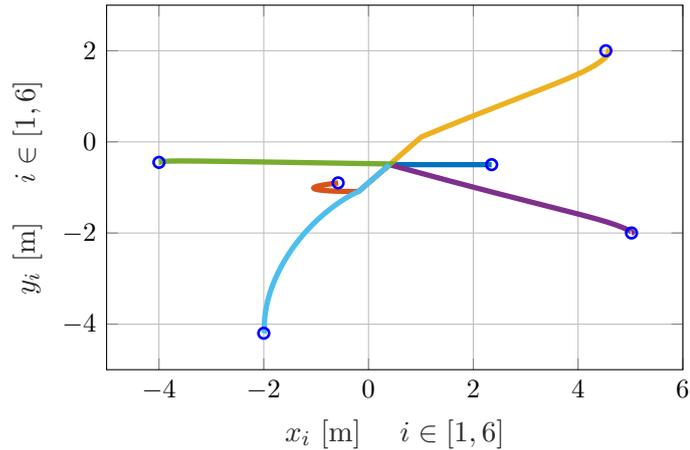
Figure 3.6: Paths described by the agents under the control law (3.82). The circles denote the initial positions.
