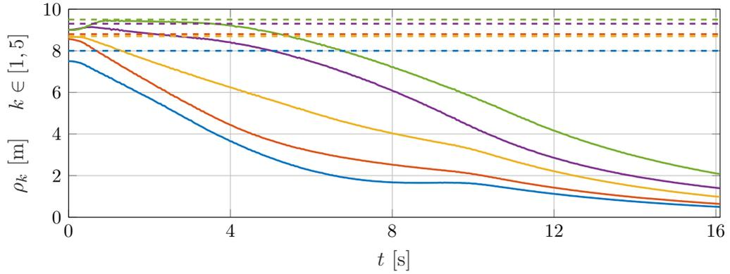
Figure 4.12: Inter-agent distances under the action of control laws (4.40)-(4.41). The dashed lines represent the range limitations.
