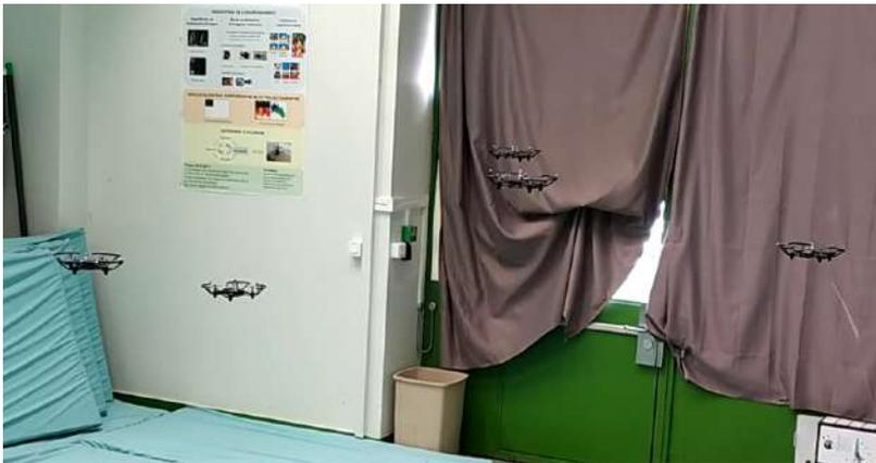
Figure 6.16: Snapshot of the experimental test using five DJI Tello EDU<sup>®</sup> drones.
