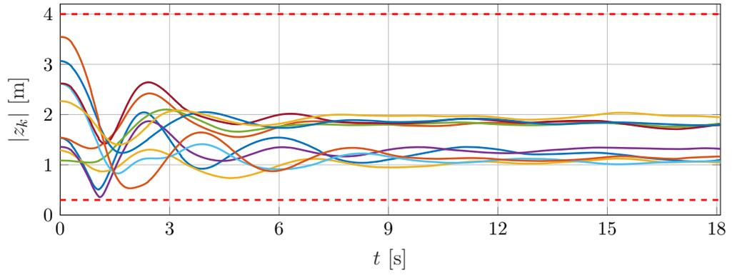
Figure 6.31: Inter-agent distances. The dashed lines represent the maximal and minimal distances guaranteeing connectivity maintenance and collision avoidance.
