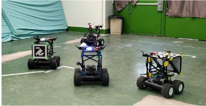
Figure 4.15: Snapshot of the experimental test using four Nexter Robotics' Wifibots.
