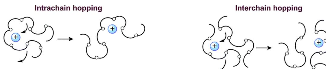
**Figure 1.9.** Illustration of ion transport in polymer matrices involving intra- and interchain ion hopping assisted by segmental motions of polymer chains. Ion-coordinating moieties along the chains are represented by open circles. Image from ref. <sup>32</sup>.
