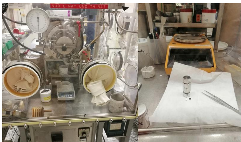
Figure 50: Left: Calcination furnace for the interaction tests between UO_2 and sodium. Right: detailed view of the capsule before the interaction test.
