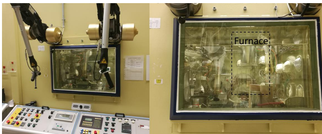
Figure 40: Left: Minor actinides cell equipped with tele-manipulators. Right: view of the calcination furnace for MOX and sodium interaction studies.
