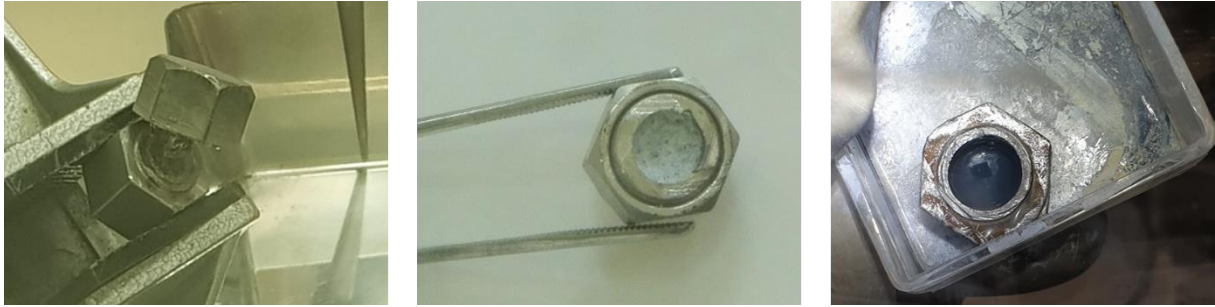
Figure 52: View of a cut capsule after the interaction. Due to the tightness, the capsule was cut by saw. Left: capsule fixed on the support for the cut. Middle: view of the excess of sodium after the interaction. Right: dissolution of the sodium excess with Ethanol.
