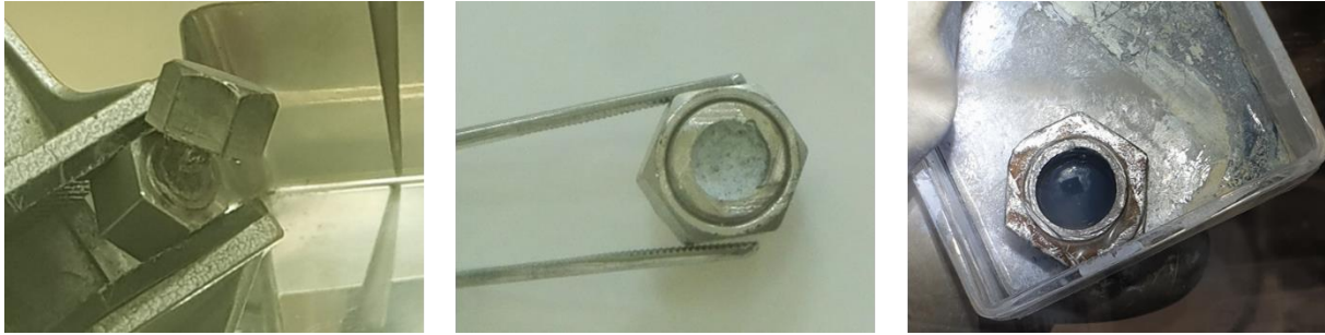
Figure 52: View of a cut capsule after the interaction. Due to the tightness, the capsule was cut by saw. Left: capsule fixed on the support for the cut. Middle: view of the excess of sodium after the interaction. Right: dissolution of the sodium excess with Ethanol.
