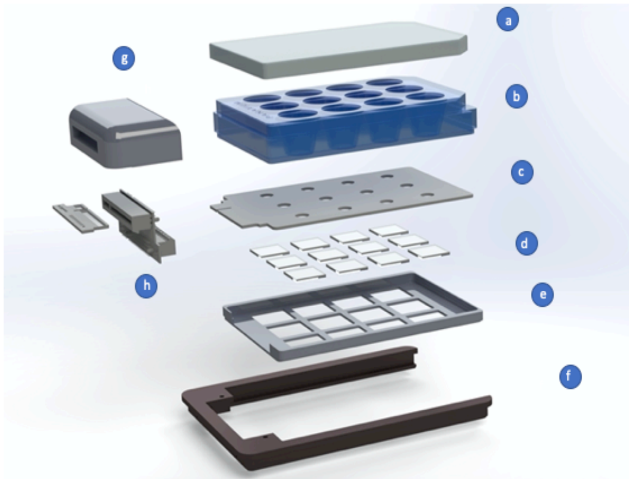
Figure 17: Solidwork rendering of the smart well plate. Exploded view of the structures displays the different components. From top to bottom: the lid, cell restrictive environment top part. The PCB and its MEA supported by the bottom part of the smart well plate. And the holder with its additive PCB and cap as g) and h).
