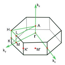
Figure 1.4: First Brillouin zone of bulk h-BN (3D lattice) with 8 critical points:  $\Gamma$ , M, K, A, L, H, K' and M'.
