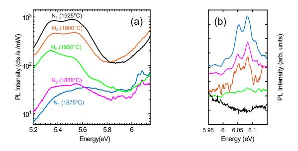
Figure 3.20: Photoluminescence spectroscopy of h-BN epilayers at 8 K: (a) raw PL data plotted in a semi-log scale. The spectra are not vertically shifted; (b) after subtraction of the laser diffusion. The spectra are vertically shifted. The samples are grown with five different MBE boron source temperatures  $T_B : N_1 : 1875^{\circ}C, N_2: 1888^{\circ}C, N_3:1900^{\circ}C, N_4: 1925^{\circ}C$  and  $N_5: 1950^{\circ}C$ . The surface morphology of these samples is presented in figures 3.9.
