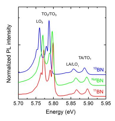
**Figure 1.13:** PL emission of h-BN at cryogenic temperature: for samples purified isotopically:  ${}^{10}BN$  and  ${}^{11}BN$  and  ${}^{Nat}BN$ .
