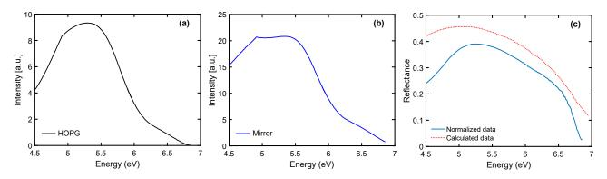
Figure 2.10: Normalization of our reflectance spectra (a) Intensity of the reflected signal from the surface of a HOPG sample as a function of energy; (b) intensity of the reflected signal from the surface of reference mirror as a function of energy; (c) Normalization of  $\frac{I_r(\lambda) \times R_{ref}(\lambda)}{I_{ref}(\lambda)}$  in solid blue line compared with the calculated reflectance of graphite (dotted red line).
