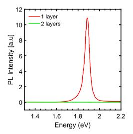
Figure 3.1: Direct band gap in monolayer  $MoS_2$ : PL spectra for mono- and bi-layer  $MoS_2$  samples in the photon energy range from 1.3 to 2.2 eV. These data are taken from Ref.[2] and they were measured at room temperature for an excitation energy at 2.33 eV.
