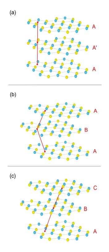
Figure 1.2: Allotropes of Boron Nitride: schematic diagrams presenting (a) the crystalline structure of hexagonal BN (h-BN) in AA' stacking; (b) the crystalline structure of bernal BN (b-BN) in AB stacking; (c) the crystalline structure of rhombohedral BN (r-BN) in ABC stacking. The red lines joining the centers of  $B_3N_3$  hexagons highlight the periodic stacking of the different structures. In all schemes: yellow spheres are Boron atoms and blue spheres are Nitrogen atoms.
