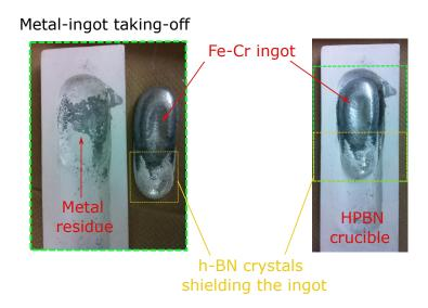
Figure 2.13: Hot-Pressed BN (HPBN) boat crucible for h-BN crystal growth: this crucible is used in the metal flux method with a temperature-gradient cooling process (left-side); Metal-ingot taken off from the crucible (right-side); both pictures show the h-BN crystals covering the metal-ingot.
