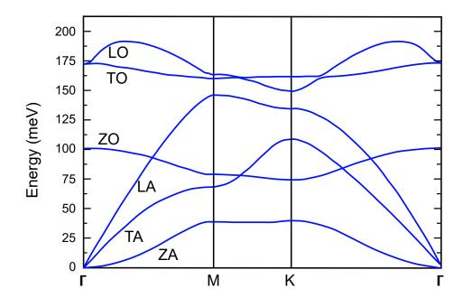
Figure 1.10: Phonon dispersion relation of mBN: calculated using local density theory (*LDA*) by Wirtz *et al.* [48].
