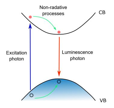
Figure 2.11: Principle of photoluminescence spectroscopy for semiconductors.
