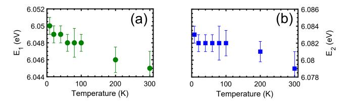
Figure 3.28: Temperature dependence of the emission in mBN: (a) spectral position of  $L_1$ ; (b) spectral position of  $L_2$  versus temperature of the sample. Error bars in both figures indicate the uncertainty on the extracted data.
