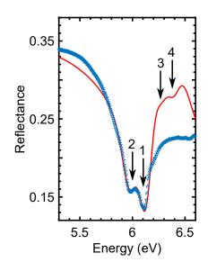
Figure 3.33: Fit of the reflectance spectrum in mBN taking into account 4 Gaussian distributions centered at  $\Omega_1 = 6.12 \text{ eV}$ ,  $\Omega_2 = 5.98 \text{ eV}$ ,  $\Omega_3 = 6.29 \text{ eV}$  and  $\Omega_4 = 6.39 \text{ eV}$ : inhomogeneous broadening  $\sigma = 76 \pm 2 \text{ meV} >>$  homogeneous broadening  $\hbar\Gamma = 35 \pm 1 \text{ meV}$ ,  $\eta_{min}^{(1)} = 100\%$ ,  $\eta_{min}^{(2)} = 50 \pm 2\%$ ,  $\eta_{min}^{(3)} = 30 \pm 2\%$  and  $\eta_{min}^{(4)} = 20\%$ .
