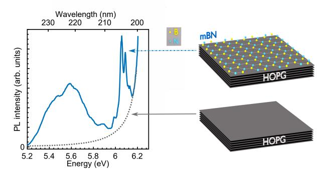
Figure 3.14: Photoluminescence of epitaxial monolayer BN on graphite: leftside: in blue solid line is the PL spectrum recorded from mBN; in dotted grey line is the signal recorded from HOPG; both spectra are recorded at 8K, with a laser excitation of 6.375 eV (194.47 nm); right side: schematics of the mBN-graphite heterostructure synthesized by van-der-Waals epitaxy, and HOPG substrate. HOPG stands for highly oriented pyrolytic graphite.
