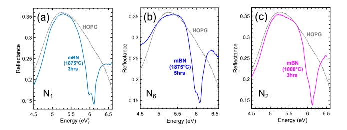
Figure 3.24: DUV reflectance spectrum for several mBN samples measured at 8 K, obtained for different MBE boron cell temperatures  $(T_B)$  and growth times: (a)  $T_B$ =1875°C, 3 hours, (b)  $T_B$ =1875°C, 5 hours, (c) TB=1888°C, 3 hours. The solid grey line is the reflectance spectrum of the bare HOPG substrate for reference.
