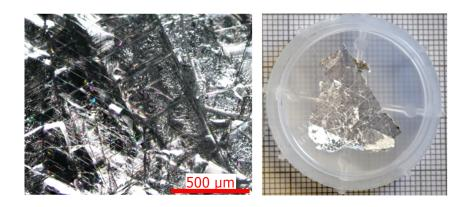
Figure 2.14: h-BN bulk crystals grown by metal flux method: on the left side is an image taken by an optical microscope; on the right side is a macro image of the peeled h-BN flake with a size of about 3 cm placed in the wafer carrier.
