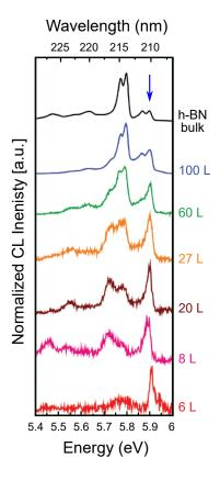
Figure 3.3: Variation of the emission spectrum of h-BN as a function of the number of layers: CL spectra measured at 8K from bulk h-BN and flakes of 100, 60, 27, 20, 8 and 6L. The blue vertical arrow shows the position of the LA-TA phonon replicas in the emission spectra of h-BN. These data are taken from Ref. [84].
