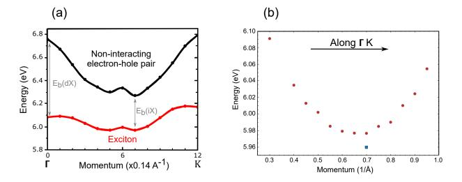
Figure 1.9: Dispersion of excitons in h-BN: (a) dispersion of excitons in h-BN compared to the noninteracting electron-hole pair along the  $\Gamma K$  line, with the momentum q corresponding to CM. The vertical arrows indicate the binding energy  $E_b$  for the direct (dX) and indirect (iX) excitons [43]; (b) dispersion energy of the fundamental exciton in bulk h-BN along  $\Gamma K$  direction, determined from EELS (*Electron Energy Loss Spectroscopy*) measurements [44].
