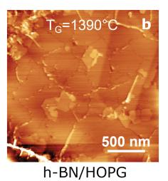
Figure 3.6: Atomic force microscopy images of h-BN by MBE at high temperature: (a) AFM image of h-BN grown on sapphire; (b) AFM image of h-BN grown on HOPG. Both samples were grown for 3 h, at  $T_G=1390^{\circ}$ C and a boron cell temperature  $T_B=1875^{\circ}$ C. These data are taken from Ref.[67].
