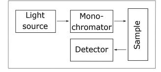
Figure 2.2: Configuration used to build our reflectance experiment: The light emitted by the source is filtered spectrally by a monochromator before reaching the sample surface. The reflected light from the sample surface is directly detected by a photo-detector.
