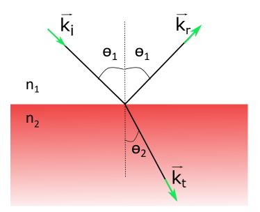
Figure 2.1: Schematic plot showing partial reflection, and refraction of an electromagnetic wave with a linear polarization at an interface between two different media:  $\theta_1$  is the angle between the normal and the incident/reflected wave in the medium (1);  $\theta_2$  is the angle between the normal and the refracted wave in the medium (2);  $\vec{k}_{i,r,t}$  are the corresponding wave-vectors.
