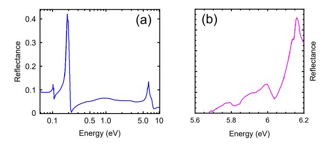
Figure A.1: Reflectance of BN: (a) Reflectance spectrum measured from pyrolitic BN at room temperature. These data are taken from Ref. [128]; (b) Reflectance measurements from high quality h-BN at 8K. These data are taken from Ref. [129].
