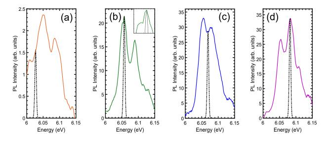
Figure 3.18: PL emission of mBN for different values of the excitation energy: data are plotted after subtraction of stray laser light; the excitation energies are  $E_{ex}$ : (a) 6.345 eV; (b) 6.375 eV, (c) 6.39 eV, (d) 6.4 eV; Rayleigh scattering of the laser is plotted in black dotted lines and shifted by the Raman energy  $2\Delta$ , with  $\Delta = 159$  meV, corresponding to the energy of the LA(M) phonon in mBN.
