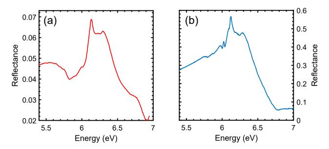
Figure A.2: Reflectivity of bulk h-BN (a) Reflectivity spectrum measured from bulk h-BN crystal from HQgraphene company at 8K using a Deuterium lamp as a light source; (b) Reflectivity spectrum measured from bulk h-BN crystal from Kansas University at 8K using a Xenon-plasma light source. Both spectra are normalized following the procedure described in chapter 2, section 2.1.1 using the same reference mirror.
