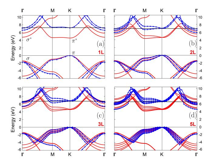
Figure 3.2: Calculations showing the variation of the band structure for h-BN as a function of the number of layers: (a) for monolayer; (b) for bilayer; (c) for trilayer and (d) for pentalayer. The band extrema for monolayer are situated at the K point of the first Brillouin zone (BZ). For the number of layers higher than 2, the band extrema are situated along the MK direction [8].
