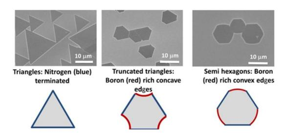
Figure 3.4: Shape dependence of the h-BN grains on the growth conditions: first line: SEM images of the h-BN domains grown at 1065°C by CVD method on Cu foils; second line: Sketch of the resulting h-BN crystal shapes and corresponding to N-termination in blue and B-termination in red. Form left to right the N:B ratio was decreased during the growth. These figures are taken from Ref. [91].
