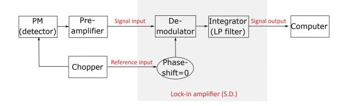
Figure 2.5: Principle of synchronous detection: scheme resuming the process of synchronous detection in our setup with a phase shift chosen to maximize the modulated signal.
