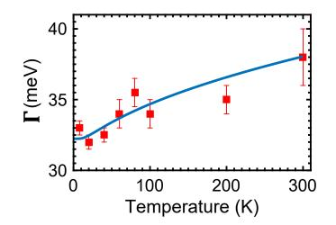
Figure 3.30: Temperature dependence of the emission in mBN: variation of full width at half maximum  $\Gamma$  for the lines in the PL doublet as a function of the temperature of the sample (From 8K to 300K); extracted parameters are shown in symbols and the fit is shown in blue solid line.
