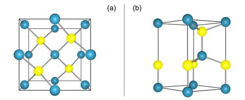
Figure 1.1: Allotropes of Boron Nitride: (a) schematic diagram presenting the crystalline structure of cubic BN (c-BN); (b) schematic diagram presenting the crystalline structure of wurtzite BN (w-BN). In both schemes: yellow spheres are Boron atoms and blue spheres are Nitrogen atoms.
