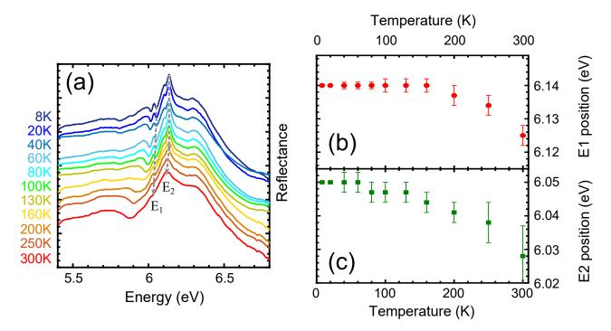
Figure A.4: Reflectance spectra in bulk h-BN as a function of temperature (a) Reflectance for different temperatures of the sample. For each spectrum we indicate the temperature on the left side; (b) Variation of the energy position  $E_1$  indicated in panel (a); (c) Variation of the energy position  $E_2$  indicated in panel (a).
