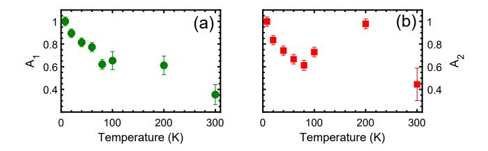
Figure 3.29: Temperature dependence of the emission in mBN: (a) normalized amplitude  $A_1$  versus temperature of the sample; (b) normalized amplitude  $A_2$  versus temperature of the sample. Error bars in both figures indicate the uncertainty on the extracted data.
