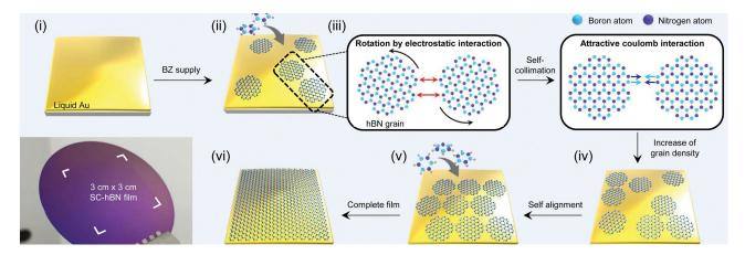
Figure 3.5: Growth of h-BN single layer on the surface of a molten Au: Schematic illustration for the growth of h-BN film by means of circular h-BN grains with a rotation invoked by the attractive Coulomb interaction of B and N edges between grains (i to vi). And a photograph of the wafer-scale h-BN film on a SiO<sub>2</sub>-Si wafer. This figure is taken from Ref. [89].
