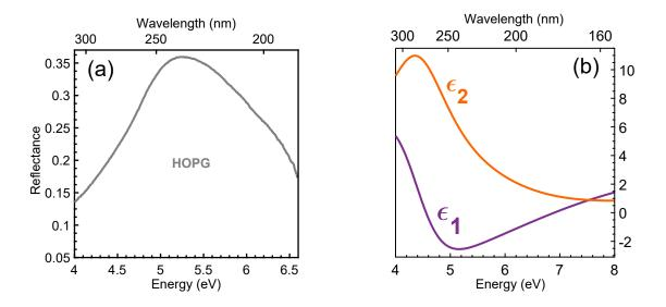
Figure 3.22: Optical response of graphite in the DUV (a) reflectance spectrum in the deep ultraviolet for the bare graphite substrate, measured at 8K, under nitrogen environment and using Deuterium lamp; (b) real ( $\epsilon_1$ ) and imaginary ( $\epsilon_2$ ) parts of the dielectric permittivity of graphite: these data are taken from ref. [66].
