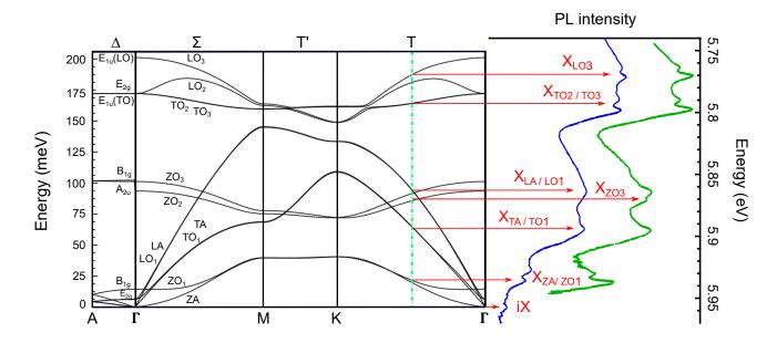
Figure 1.12: PL emission of h-BN at cryogenic temperature: (right side) PL spectra of bulk h-BN [59, 60] plotted at the same scale as the phonon dispersion relation [53] (left side); the energy of the indirect exciton (iX) coincides with the zero-phonon energy.
