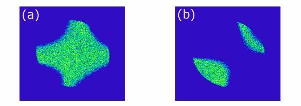
Figure 2.7: Illumination diagrams after the exit slit of the monochromator simulated using Zemax: (a) result of the simulation for slit width of about  $30\mu m$ ; (b) result obtained for slit width of  $150\mu m$  and by adding to the previous simulation a tiny off-center misalignment at the input slit of the monochromator.
