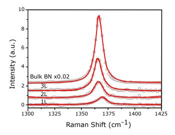
Figure 3.7: Raman spectra of atomically thin BN: Dependence of the Raman spectra on the thickness of h-BN exfoliated layers. The layers have been deposited on  $SiO_2/Si$  substrate. These data have been measured using a green laser with an excitation wavelength of 514.5 nm. The data are taken from Ref.[50].
