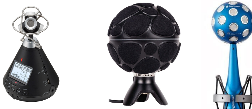
Figure 2.1: Examples of microphone arrays suitable for the encoding of the recorded sound field into the Ambisonics format. Left: Zoom’s H3-VR (4 capsules, Ambisonics format up to order 1); middle: Zylia’s ZM-1 (19 capsules, up to order 3); right: mh acoustics’ EigenMike (32 capsules, up to order 4).
