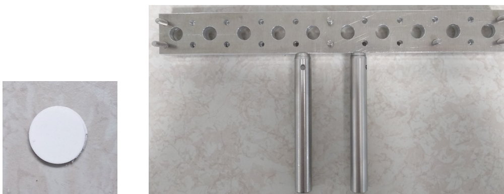
FIGURE 1.19: A pellet - disc composed of pressed powder - on the left, and its holder on the right. The holder was designed with Solidworks and built with aluminum in the laboratory workshop.
