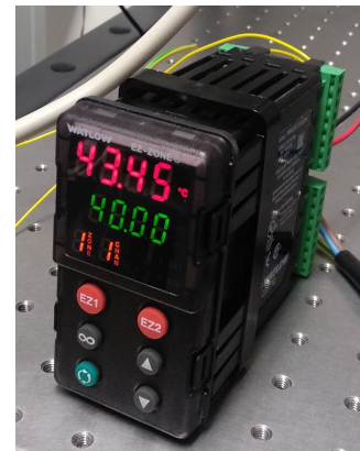
(C) Picture of the PID controller. In red is the current measured temperature and in green is the temperature setpoint to reach.
