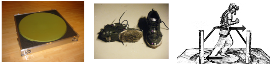
Figure 2.12 – Low-friction surfaces devices. Left and Center: the Wizdish ( Swapp et al. 2010 ). Right: the Cyberith Virtualizer ( Cakmak and Hager 2014 ).
