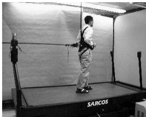
Figure 2.9 – Example of linear treadmills : the Sarcos treadport (Hollerbach et al. 2000).
