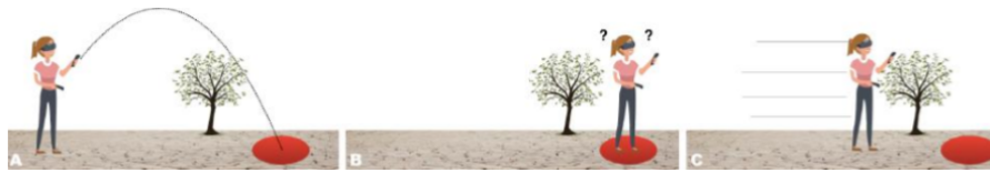
Figure 2.17 – New solution of teleportation based on continuously moving the user to the destination (A to C) instead of discontinuously translates the user’s viewpoint over a distance (A to B) (Bhandari et al. 2018).
