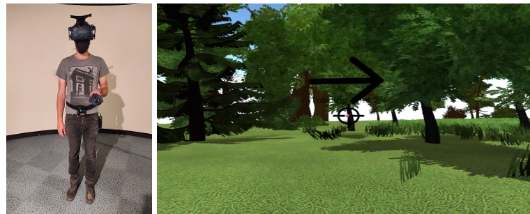
Figure 8.1 – Left - User wearing the HTC Vive Pro Eye HMD equipped with a wireless module, one HTC Vive tracker located at the pelvis and one HTC Vive controller. Right - User’s point of view of the VE during the experiment. The black arrow indicates the direction of the turn. The sight and pink sphere were used for calibration purposes).
