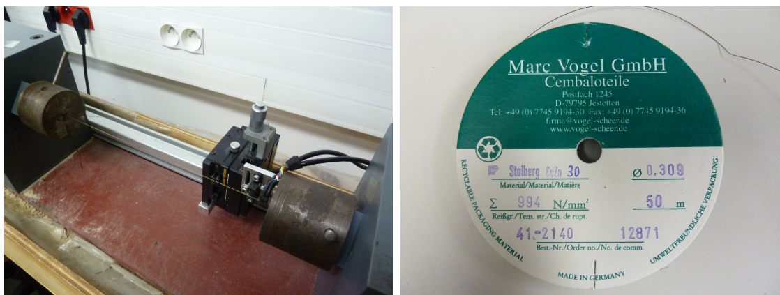
Figure 3.1: String bench used to measure the damping of the studied strings by means of optical forks (left), String made of copper and zinc by Vogel used to study the damping of the studied strings (right)
