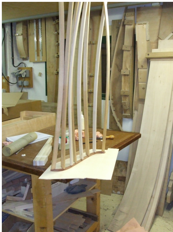
Figure 8.4: Gluing of the soundboard with the bridge of the LAM1 clavichord designed by Dancet and Ducornet during its construction.
