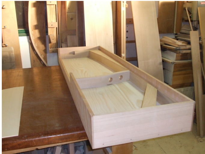
Figure 8.5: Box of the LAM1 clavichord designed by Dancet and Ducornet during its construction.
