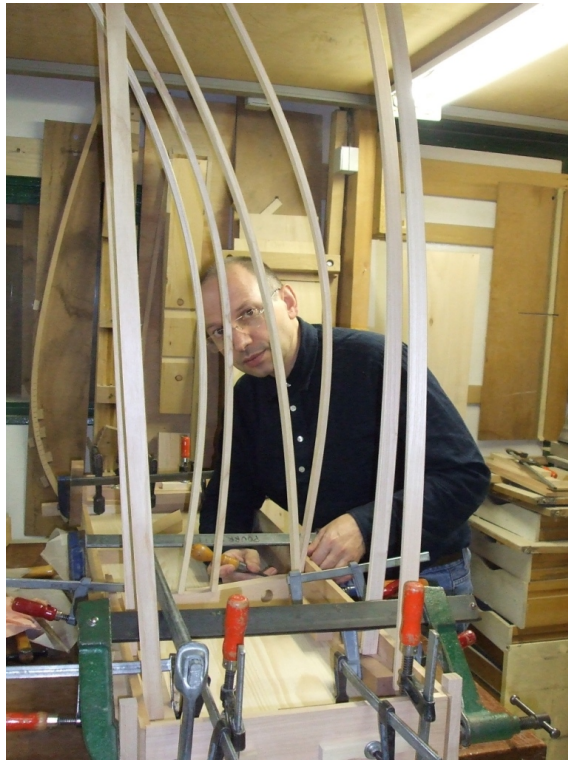
Figure 8.3: Building of the LAM1 clavichord box.
