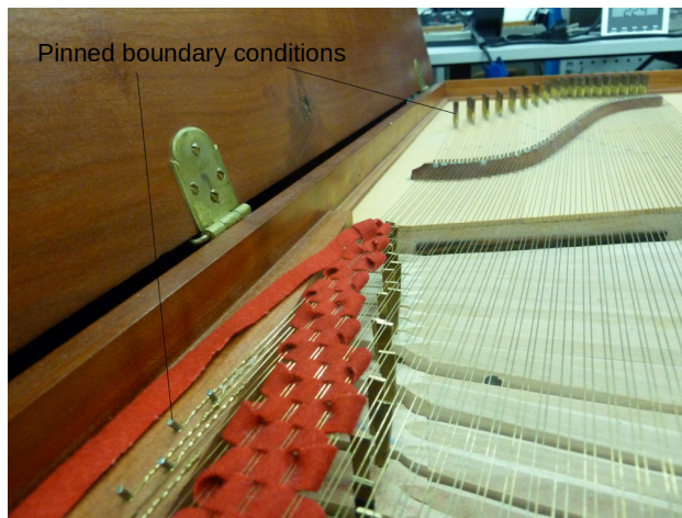
Figure 4.1: Photo indicating the pinned nature of the boundary conditions of clavichord strings
