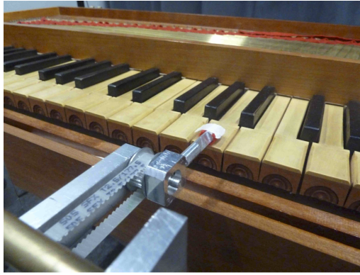
Figure 5.5: DRoPiC robotic finger for key trajectory control.
