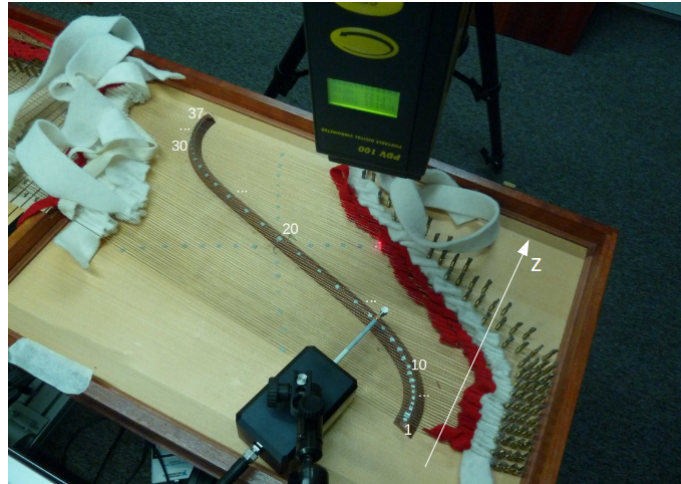
Figure 8.6: Experimental setup for the modal analysis of the bridge, with the designation measurement point number, with the z axis.
