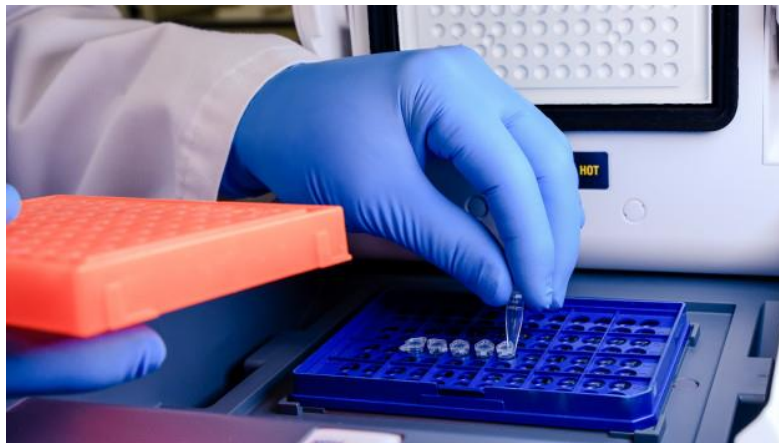
Figure 66. Picture showing an open thermocycler. The samples inside the PCR microtubes are heated at the level of their caps when the upper part of the thermocycler (in white on the picture) is shut onto the tubes.
