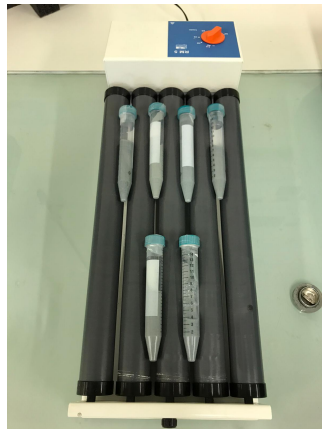
Figure 4.3: Zinc suspensions under continuous mixing using a tube roller mixer.
