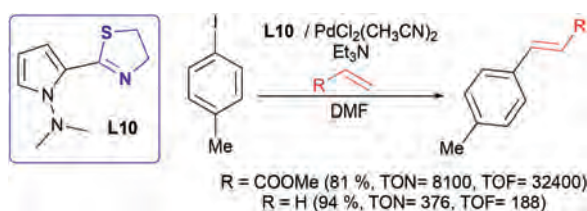
Scheme 42 Pyrrolic bidentate ligand L10 used as a catalyst in the Mizoroki–Heck reaction of aryl iodides with methyl acrylate under microwave irradiation. 82
