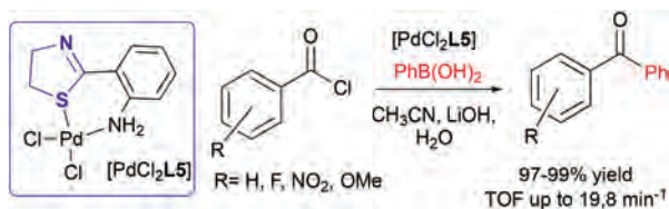
Scheme 38 [\text{PdCl}_2\text{L5}] complex-mediated coupling reaction of acid chloride with arylboronic acids. 78,79
