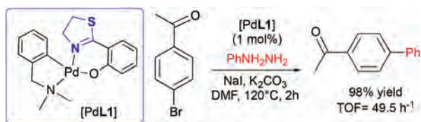
Scheme 37 Pd complexes bearing L1 ligand catalyzed cross-coupling reaction of 4-bromoacetophenone with phenylhydrazine. 76
