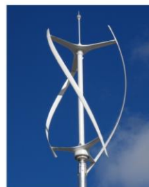
THE q5 QuietRevolution wind turbine The q5 was designed in response to increasing demand for wind turbines that work well in environments close to people and buildings. The elegant helical (twisted) design of the q5 ensures a robust performance even in turbulent winds. It is also responsible for virtually eliminating noise and vibration. At five metres high and three metres in diameter, it is compact and easy to integrate, and with just one moving part, maintenance can be limited to an annual inspection.
