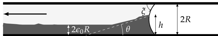
Figure 4.5: Bulldozing onset. The liquid is slowly withdrawn out of the tube at a constant flow rate. The meniscus at the air-liquid boundary can bulldoze the particles resting in the sedimented layer of height 2\epsilon_0 R , forming a particles front of height h .
