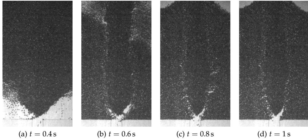
Figure 3.11: Discharge of the silo with a flat opening for the highest magnetic field amplitude  $\Psi = 62$ . The grains at the centre of the chamber do not move and the granular flow stops after one second.
