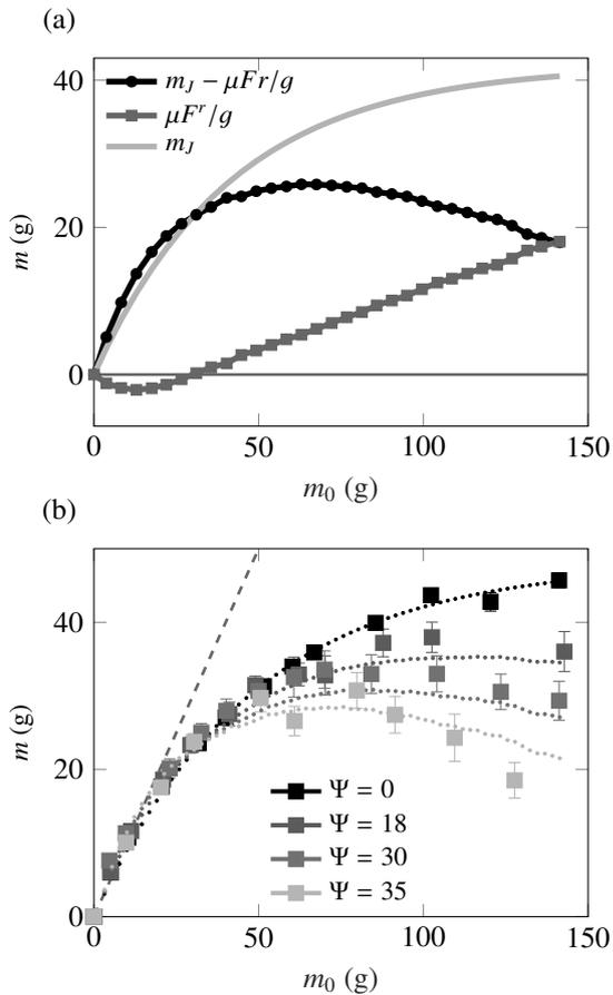
**Figure 4.** (a) Model curves for a vertical magnetic field. The light grey line shows the classical Janssen prediction; the grey squares line is the result of the computed magnetic mass loss  $\mu F^r/g$ ; the black circles line (difference of both curves) gives the predicted apparent mass of the column. (b) Comparison of the model to the experimental data points.
