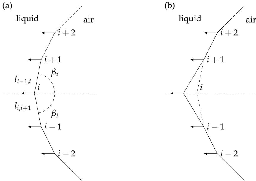
Figure 4.12: Meniscus simulation. (a) The meniscus is simulated as a point assembly where the local curvature is computed using the local angle  $\beta_i$  and points distances  $l_{i,i+1}$ . (b) At each time step the point of lower local pressure advances normal to the meniscus over a distance  $\delta l$ .
