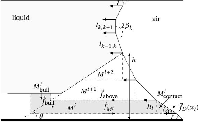
Figure 4. Global sketch of the simulated system. First, the meniscus is modelled by a series of points  $k$  characterised by the pair distances  $l_{k,k+1}$  and local angle of curvature  $2\beta_k$ . Second, the bulldozed front, of height  $h$  and avalanche angle  $\theta$ , is cut in different layers. Each layer of mass  $M^i$  is in contact with a bulldozing part  $M_{\text{bull}}^i$  and a tilted part  $M_{\text{contact}}^i$ .
