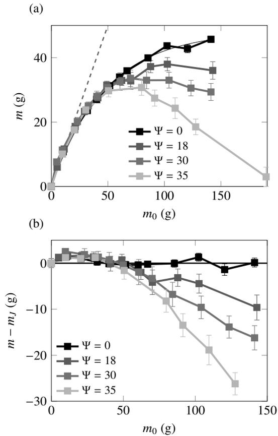
**Figure 2.** (a) Apparent mass measured using our experimental setup for different magnetic field amplitude, the black continuous line corresponds to the Janssen model  $m_J$  and the grey dashed line represents the hydrostatic limit. (b) Mass difference between the apparent mass of the system and the Janssen expression  $m_J$  for different magnetic field amplitude.
