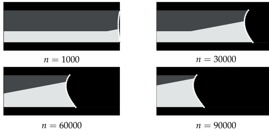
Figure 4.17: Typical example of the capillary washboarding simulation at different time steps  $n$ . 15% of isopropanol and initial amount of particles  $\epsilon_0 = 0.3$ .
