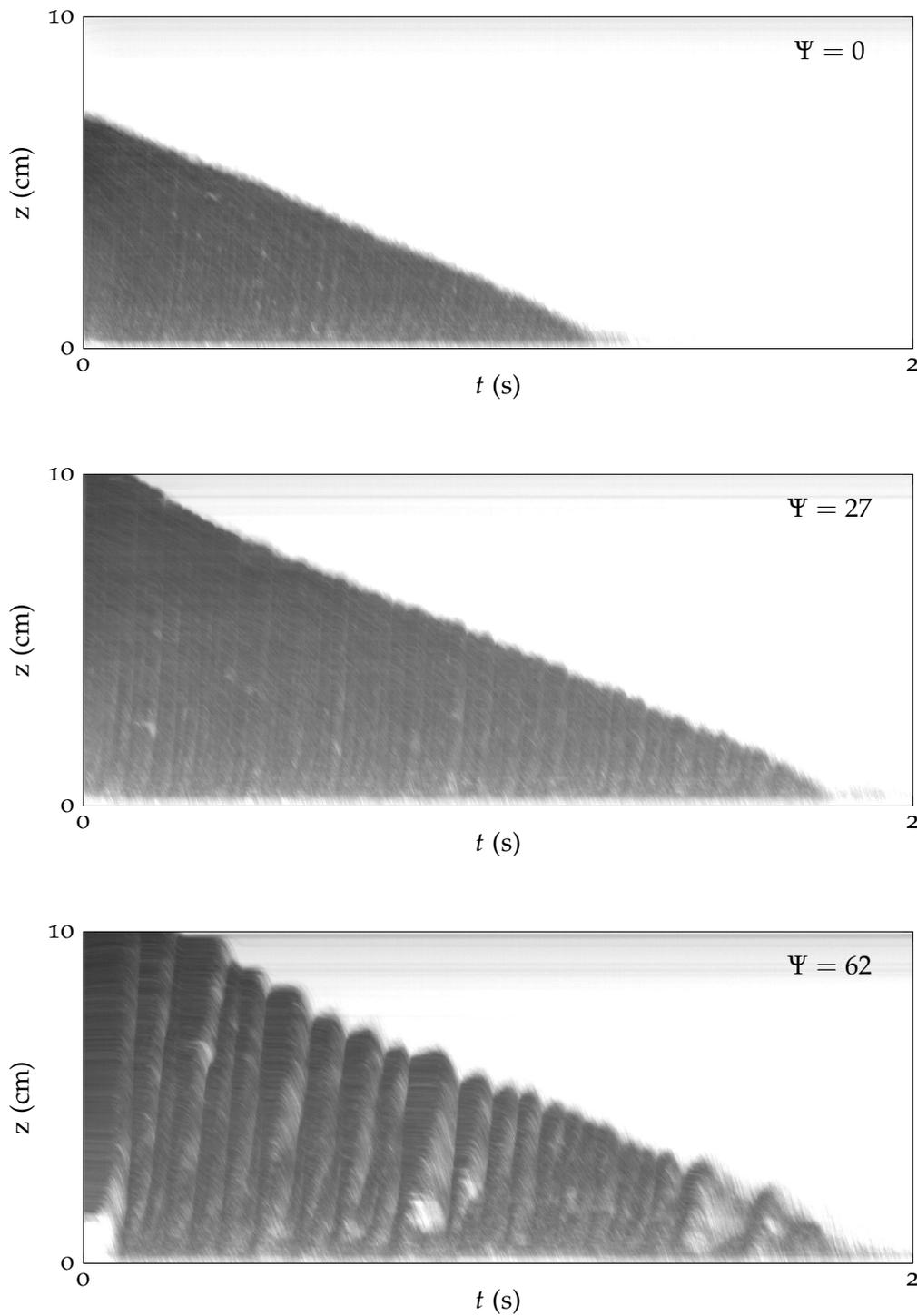
Figure 3.10: Spatio-temporal maps of the density of grains in the upper chamber for different magnetic field strength  $\Psi$ . The maps were obtained by averaging the pixel in the greyscale window above the opening at each time step. The white lines inside the granular packing correspond to the apparition of air bubbles propagating from the neck to the free surface of the packing.
