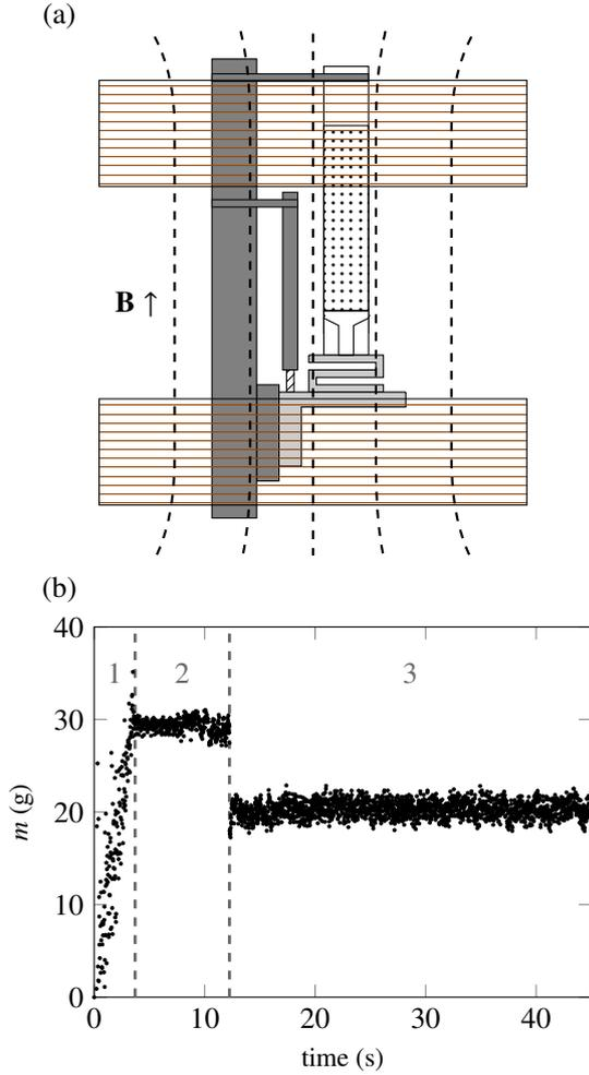
**Figure 1.** (a) Sketch of the experimental set-up with the generation of a homogeneous vertical magnetic field, using coils in a Helmholtz configuration. (b) Typical mass measurement, 1. beads are poured inside a tube using a hopper until we reach the desired mass  $m_0$ , 2. the packing is at rest and the hopper is removed, 3. downward movement of the vertical translation stage, the mass measurement corresponds to the mean plateau value.
