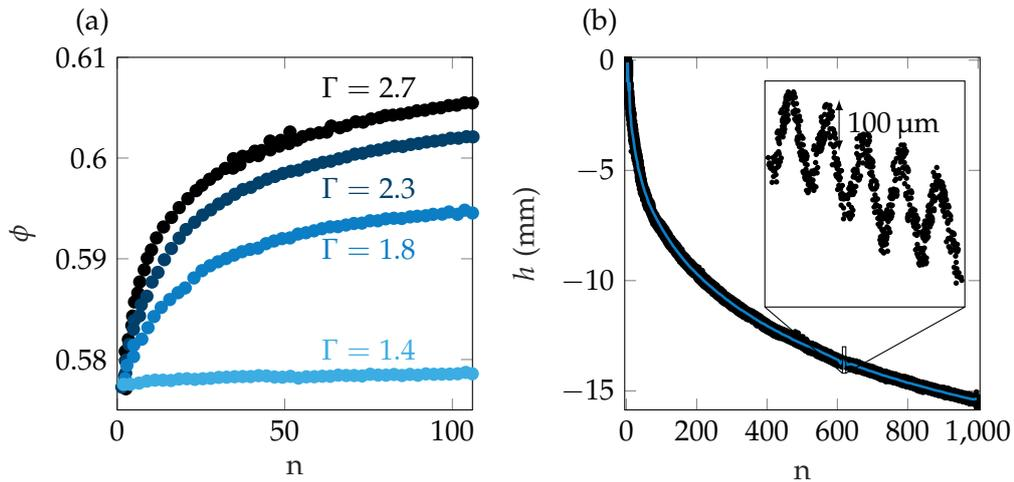
Figure 1.11: Compaction of granular material. (a) Data from [26] Mechanical compaction for different vibration intensity  $\Gamma = a/g$  where  $a$  is the tap acceleration. (b) Data from [27]. Compaction using temperature cycles of a 140 cm tall column with a temperature oscillation of  $\Delta T = 10.8 \text{ }^\circ\text{C}$  of periodicity  $2\pi/\omega = 600 \text{ s}$ .
