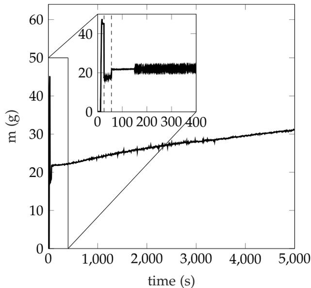
Figure 3.2: Typical aging of the granular column. The apparent mass measurement is carried on after the Janssen apparent mass estimation when friction forces are mobilized in the vertical direction (inset). The apparent mass of the granular column keeps increasing once the piston stops its downward movement.
