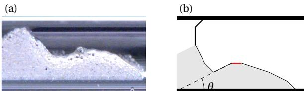
Figure 6. Descent phase of the meniscus during experiment (a) and simulation (b). When the local angle of attack is lower than a threshold  $\alpha_{\min} = 4^\circ$  (in red), the meniscus plunges in the sedimented layer of beads.
