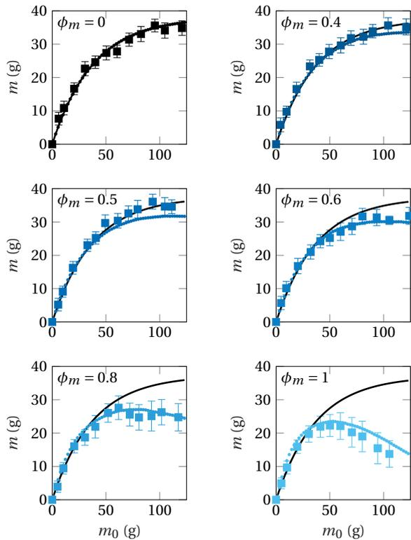
Figure 3. Mass measurement of the beads for a vertical magnetic field  $B = 170$  G and varying the magnetic fraction of the packing  $\phi_m$ . The colour squares are the experimental data, the black line represents the classical Janssen prediction while the colour dots represent the computed model. The experiments follow the Janssen prediction until  $\phi_m \approx 0.5$  where they switch to the magnetic Janssen model.
