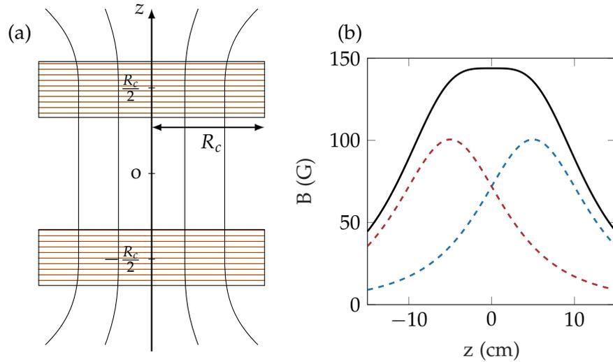
Figure 2.2: Helmholtz coils. (a) Helmholtz configuration where two identical coils of radius  $R_c$  are separated by a distance equal to their radius. (b) Magnetic field generated by the coils as the sum of both contribution and resulting in an uniform magnetic field between the two coils.
