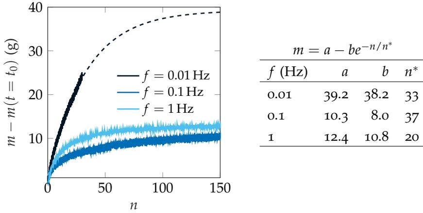
Figure 3.5: Magnetic fatigue of a granular packing for different frequency oscillations plotted against the number of magnetic oscillation cycles  $n$ . The experimental results are fitted by exponential laws (dashed lines). The fitting parameters for the different frequencies are given in the opposite table.
