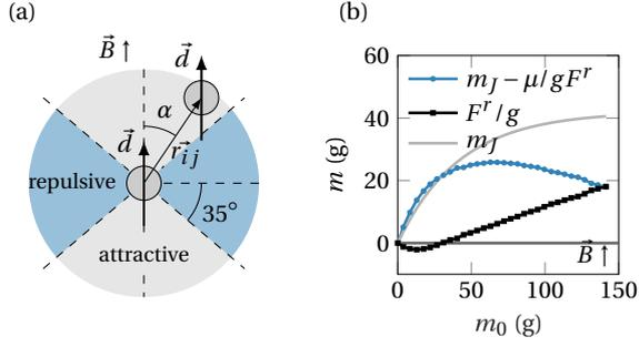
Figure 1. Magnetic Janssen effect. (a) Magnetic pair interaction between two ferromagnetic beads characterized by the magnetic moment  $\mathbf{d}$ . The interaction can be either repulsive or attractive depending on the angle between the two beads  $\alpha$ . (b) Apparent mass of the magnetic Janssen prediction for a vertical magnetic field.
