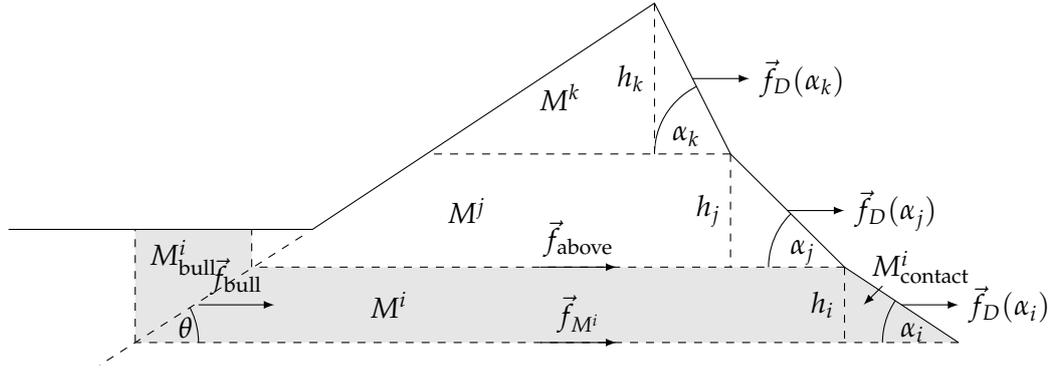
Figure 4.14: Granular packing in the simulations. The pile is divided in several horizontal layers of mass  $M_i$  in front of the meniscus planes. Each layer is bulldozing a particle front of mass  $M_{\text{bull}}^i$  and a tilted mass  $M_{\text{contact}}^i$  is in contact with the meniscus.
