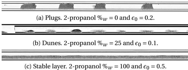
Figure 2. Different types of pattern formed along the tube depending on the liquid properties and initial height of particles. If the particles are clogging the tube, plugs are formed governed by the Janssen effect. When the meniscus is bulldozing partly the particles, a series of periodic dunes is formed on the way. For pure alcohol, the meniscus is not bulldozing any particles and the particles bed remains unperturbed.
