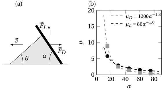
Figure 5. (a) Geometry of the pad pushed by a plane advancing at a constant velocity  $v$  with an angle of attack  $\alpha$ . (b) Data from [14]. Friction coefficients of the drag  $F_D$  and lift  $F_L$  forces.
