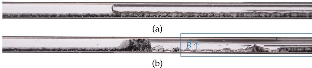
Figure 4.22: Ferromagnetic triggering of the bulldozing mechanism  $\epsilon_0 = 0.2$ ,  $\phi_m = 0.5$ . (a) No magnetic field applied, no bulldozing mechanism and the bed layer is at rest. (b) A vertical magnetic field is applied on the right side of the tube (blue zone). The bulldozing mechanism is triggered and carries on after the magnetic field is turned-off.
