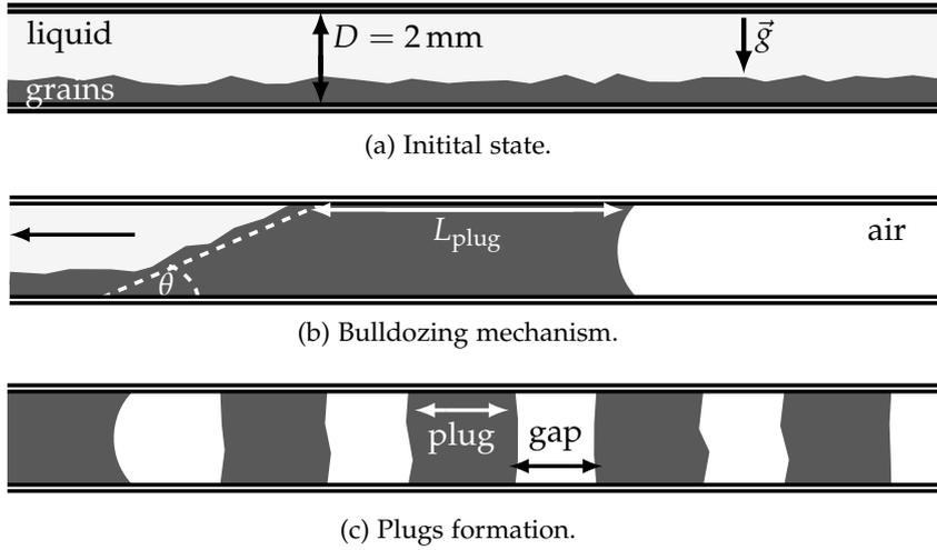
Figure 1.19: Frictional fluids in a confined geometry. (a) Initially a layer of beads is resting at the bottom and the liquid is slowly drained out of the system from one side with the other side open to air. (b) The meniscus at the liquid/air border bulldozes particles on its way. (c) After some time, the bulldozing front separates in a series of plugs along the confined geometry.
