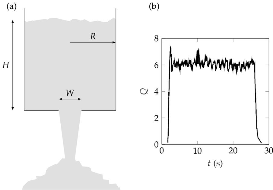
Figure 1.7: Discharge of a silo. (a) Schematic view of discharging silo characterized by its radius  $R$  and opening width  $W$ . (b) Data from [14]. Flow rate of a discharging silo, constant over time.
