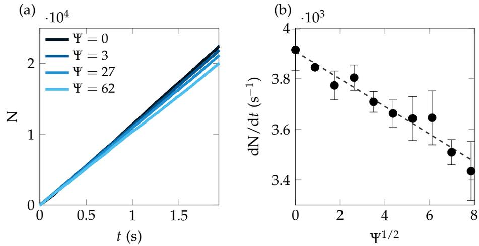
Figure 3.8: Flow rate of the discharging magnetic silo. (a) Temporal evolution of the number of particles in the lower chamber of the hourglass for different magnetic field strength  $\Psi$ . (b) Flow rate measured as the slope of the linearly increasing area of the bottom chamber.
