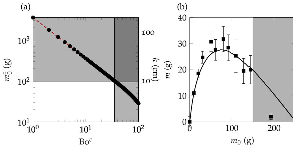
Figure 2.9: (a) Numerical computation of the critical mass  $m_0^c$ , for which the apparent mass of the packing is zero, as a function of the magnetic field strength  $\Psi$ . The grey zones represent the mass and magnetic field intensity that cannot be reached by our experimental apparatus, while the red dashed line corresponds to our theoretical prediction. (b) Apparent mass measurement for the highest magnetic field intensity, applied vertically, and comparison to our model (black line).
