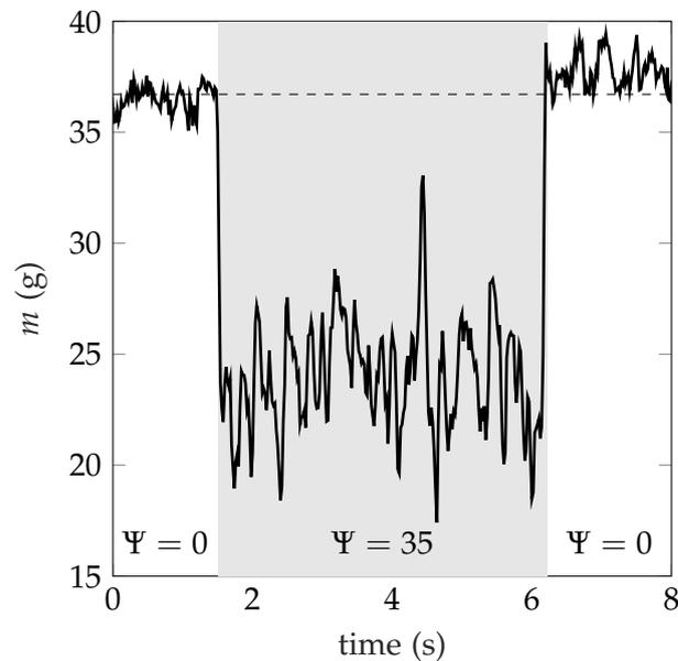
Figure 3.1: The vertical magnetic field of amplitude  $\Psi = 35$  is switched on and off during an apparent mass measurement of a column of  $m_0 = 60$  g (piston moving downward). The apparent mass jumps from the classical Janssen prediction  $m_J = 37$  g to a lower value  $m = 22$  g predicted by our "magnetic Janssen" model. When the magnetic field is turned-off again, the measured apparent mass appears slightly higher than  $m_J$ .
