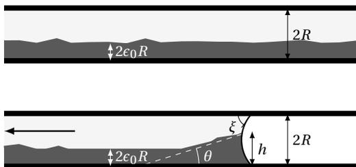
Figure 1. Bulldozing instability. A granular bed of height  $2\epsilon_0 R$  rests at the bottom of a capillary tube of height  $2R$ . While draining out the liquid out the tube, a meniscus at the liquid/air border appears. The meniscus may bulldoze partly the particles on its way forming a bulldozing front of height  $h$ .
