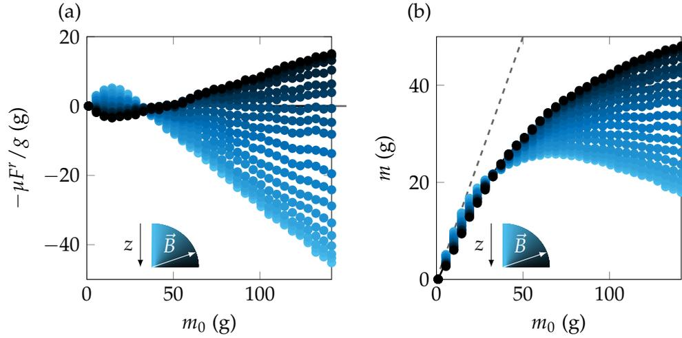
Figure 2.13: Magnetic Janssen for different magnetic field direction for  $\Psi = 35$ . (a) Global radial force contribution to the apparent mass, the contribution is zero for a magnetic angle to the vertical  $\alpha = 55^\circ$ . (b) Apparent mass of the granular column, for a horizontal magnetic field the magnetic Janssen effect is above the classical Janssen prediction.
