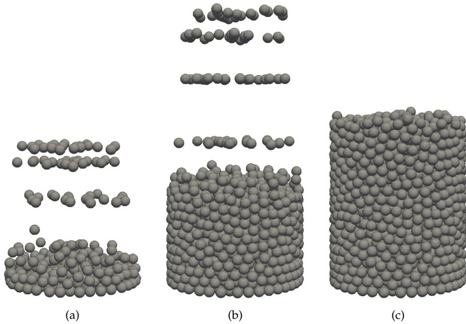
Figure 2.6: Random generation of a 3D beads packing in a geometry similar to the experiment, inspired by [61]. At each time step  $M = 20$  particles are generated at a fixed height to the top of the packing and let to sediment.
