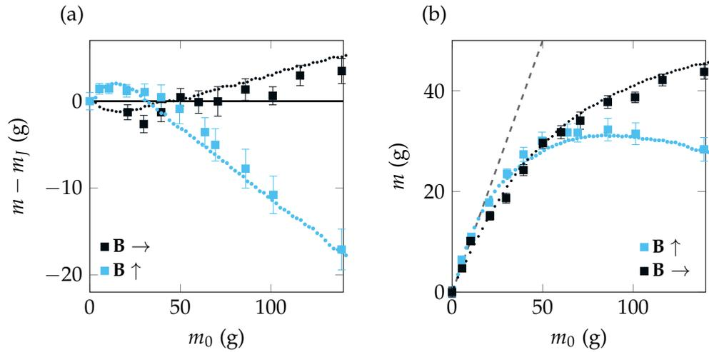
Figure 2.14: Experimental results for a vertical and horizontal magnetic field for  $\Psi = 30$ . (a) Difference between the apparent mass and the classical Janssen prediction  $m_J$ . (b) Apparent mass measurement.
