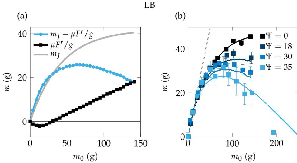
Figure 2.8: (a) Model curves, in light grey the classical Janssen prediction given by equation (1.5), in black the numerical solution for the global radial force  $F^r$ , in blue the resulting magnetic Janssen prediction given by equation (2.1). (b) Comparison of the experimental results to the magnetic Janssen prediction for a selection of magnetic Bond number  $\Psi$ . Squares correspond to the experimental results, small dots correspond to the numerical resolution.
