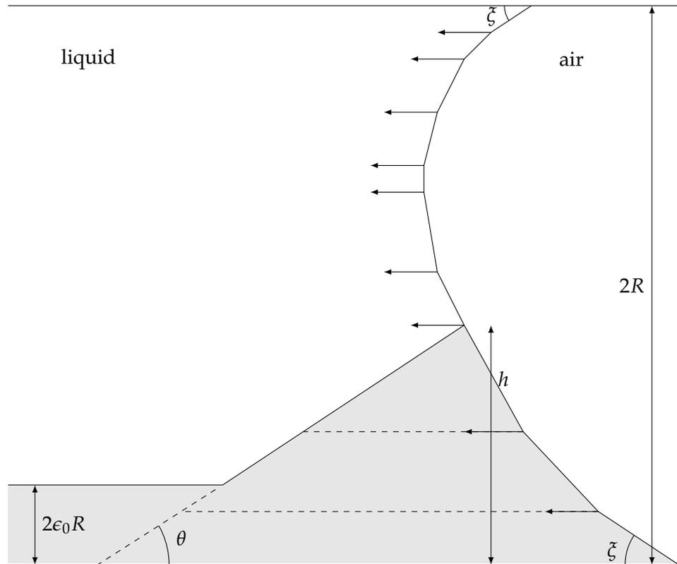
Figure 4.11: Global sketch of our simulations. The meniscus is simulated by an assembly of  $N$  points moving normally to the meniscus in contact with liquid, and in the horizontal direction when in contact with particles. At each time step we record the packing height  $h$  while the wetting conditions  $\zeta$  and the avalanche angle  $\theta$  are kept constant.
