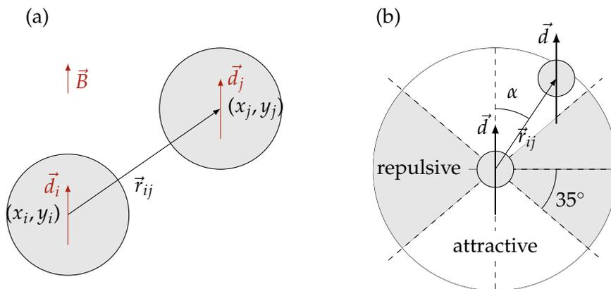
Figure 1.16: Magnetic interaction between two ferromagnetic grains. (a) When submitted to a vertical magnetic field  $\vec{B}$ , both grains acquire a magnetic moment  $\vec{d}_i, \vec{d}_j$ . (b) In the case of a uniform magnetic field, the magnetic interaction between the two beads can be either attractive or repulsive.
