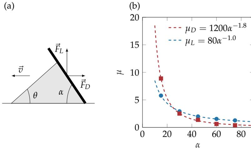
Figure 4.15: Friction pad sliding over a granular bed. (a) Geometry of the pad pushed by plane advancing at a constant velocity  $\vec{v}$  with an angle of attack  $\alpha$ . (b) Data from [74]. Friction coefficients of the drag  $\vec{F}_D$  and lift  $\vec{F}_L$  forces.
