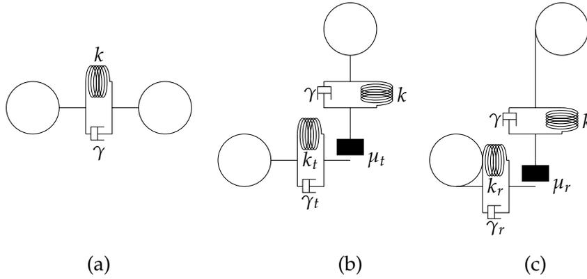
Figure 1.13: Simulation modelling of grains interactions. (a) Normal characterized by the stiffness  $k$  and dissipation  $\gamma$ . (b) Tangent characterized by the stiffness  $k_t$ ,  $\gamma_t$  and friction  $\mu_t$ . (c) Rolling characterized by the stiffness  $k_r$ ,  $\gamma_r$  and friction  $\mu_r$ .
