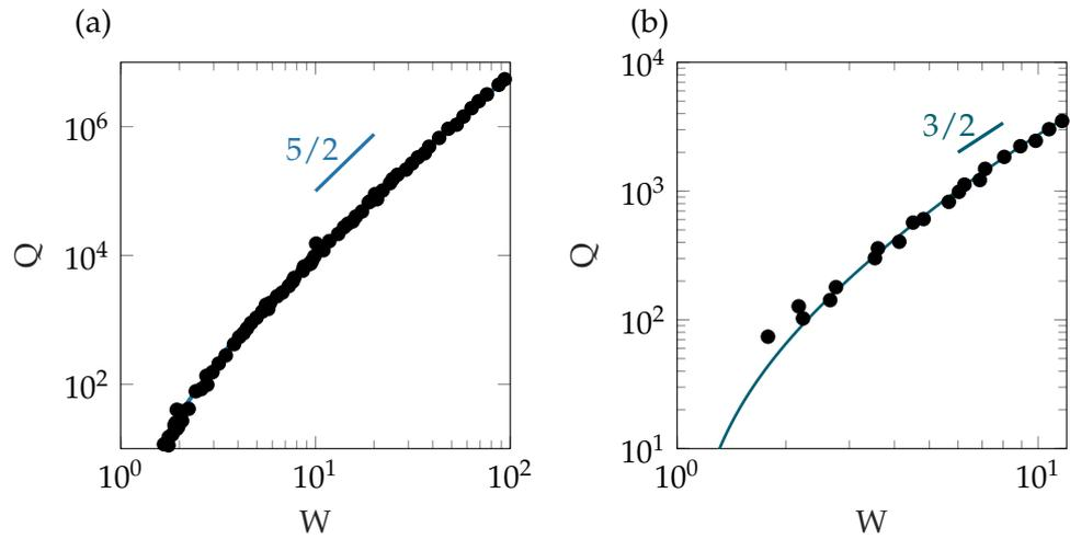
Figure 1.8: Flow rate of a discharging silo. Data from [17]. (a) (resp. (b)) Flow rate at the output of a 3D (resp 2D) silo. The experiments are following nicely the power law prediction in  $5/2$  (resp.  $3/2$ ).
