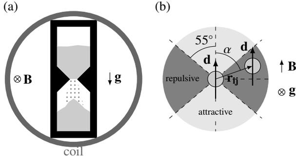
**Figure 1.** (a) Experimental setup made of a quasi 2D silo in a Hele-Shaw cell with a 45° funnel in its centre. The cell is filled with 500 μm diameter steel beads. The cell is placed in a magnetic coil generating a magnetic field perpendicular to the cell. (b) Top view of the left panel representing the dipolar interaction between two uniformly charged ferromagnetic beads characterized by the dipolar moment  $\mathbf{d}$ .
