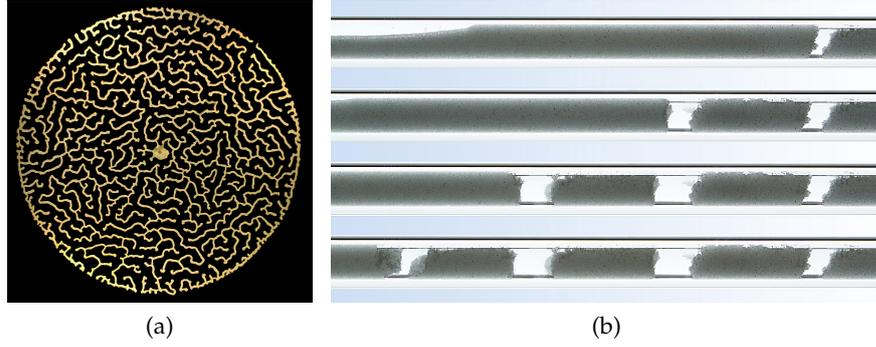
Figure 1.20: Confined frictional fluids experiments. (a) Drainage inside a Hele-Shaw cell resulting in a labyrinthine pattern [51]. (b) Drainage inside a capillary tube resulting in a series of plugs along it [52].
