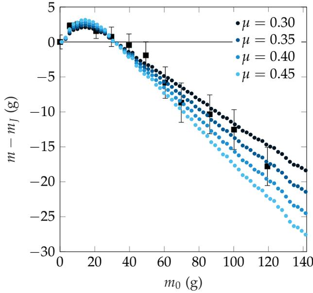
Figure 2.11: Influence of the friction coefficient. The difference between experimental data points at  $\Psi = 30$  and classical Janssen prediction  $m_J$  is compared to the numerical solution where we varied the value of the friction coefficient. The best fit is found for  $\mu = 0.35$  in this case.
