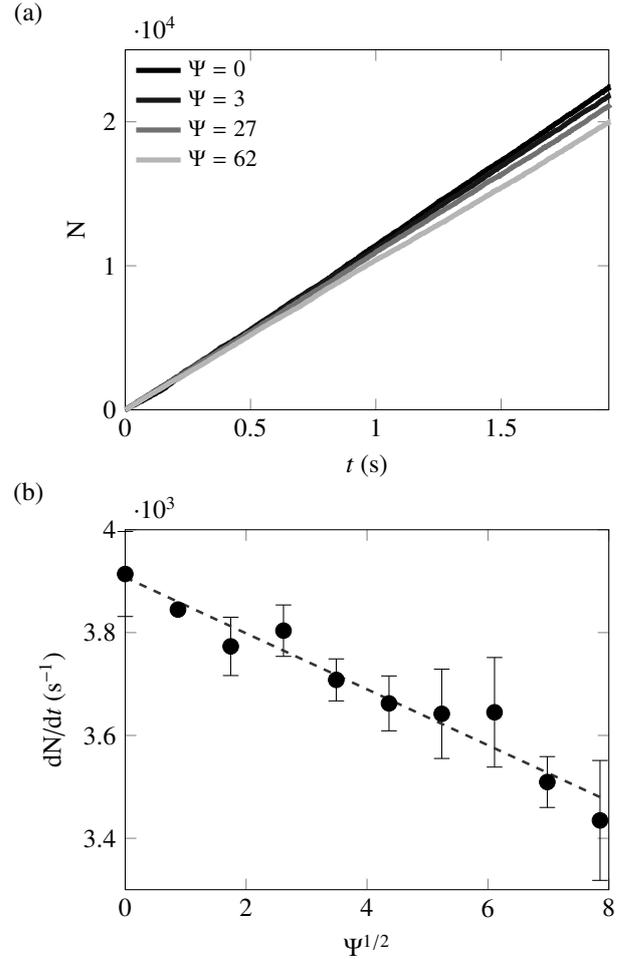
**Figure 2.** (a) Cumulative number of beads in the lower part of the cell during time for different magnetic field. (b) Flow rate of the beads in the silo given by the slope of the cumulative number of beads. The flow rate decreases when increasing the magnetic field intensity. The dashed line corresponds to a linear fit of the experimental data. Error bars correspond to the standard deviation over three realizations.
