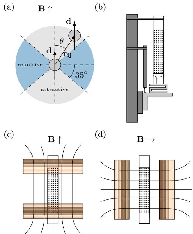
**Fig. 1 Experimental setup.** **a** Anisotropic magnetic dipolar interaction between two ferromagnetic particles subjected to the magnetic field  $\mathbf{B}$ . **b** Ferromagnetic particles fill a cylindrical tube and rest on a piston fixed to a force sensor. This piston can be displaced vertically thanks to a motorized translation stage. **c, d** The column is placed between two magnetic coils mounted in a Helmholtz vertical or horizontal configuration to create a uniform magnetic field.
