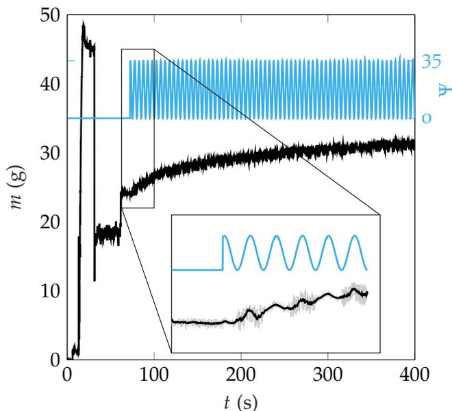
Figure 3.3: Typical magnetic fatigue of a granular column of mass  $m_0 = 60$  g. The apparent mass, in black, is measured during a Janssen effect experiment followed by a oscillating magnetic field of amplitude  $A = 170$  G and frequency  $f = 0.1$  Hz, shown in blue.
