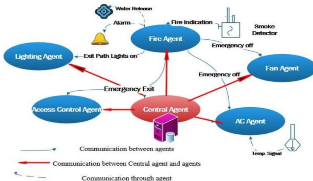
Figure 3. Example of the architecture of a multi-agent system (extracted from [Priyadarshana et al. 2017])
