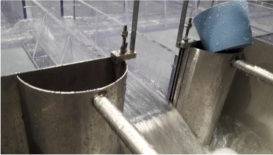
Figure 3: View of the opening of a tank of MURI acting as outlet.
