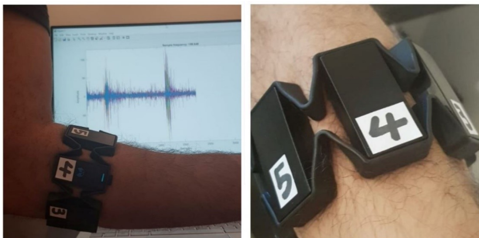
Figure 4-2 Acquisition of sEMG data of a user to create the database (Enrolment)
