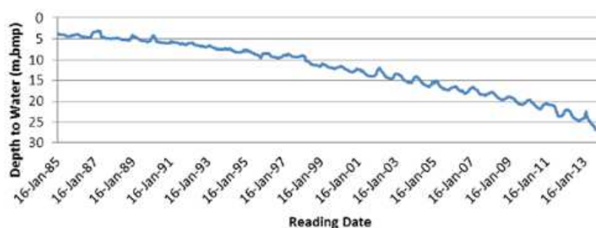
Figure 4-8. Fluctuation in groundwater table in Awsa field, Azraq (WAJ, 2014)
