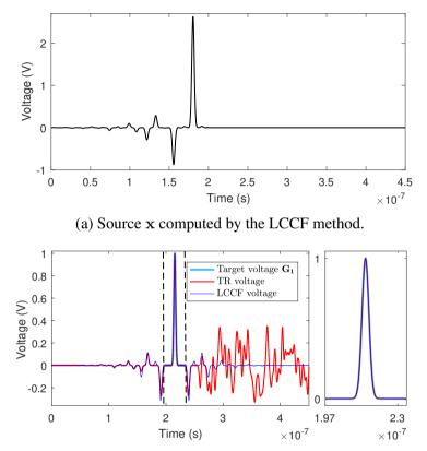
(b) Voltage signals y recorded after injecting the LCCF source x and the TR backpropagated signals.
