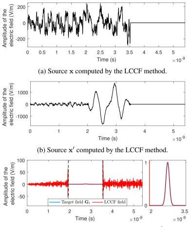
(c) Electric signal y recorded by R after injecting x and x' simultaneously.
