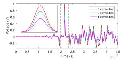
Figure 2.11: During separate TR processes in a lossless network, not considering all the absorbent extremities causes information losses and leads to an improper refocusing of  $\mathbf{G}_1$ . The small figure represents the signals zoomed over the refocusing time  $[1.95 \times 10^{-7}, 2.34 \times 10^{-7}]$ .
