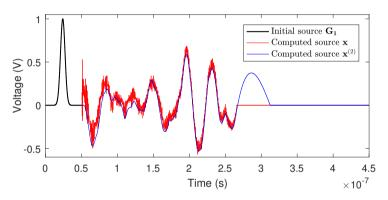
(b) Composed source  $\mathbf{G}_1 + \mathbf{x}_{160 \rightarrow f}$  before and after *a priori* filtering.
