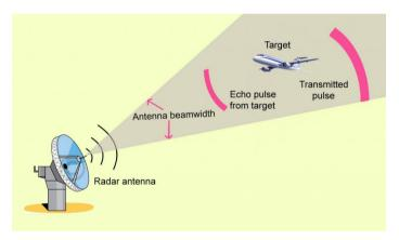
Figure 1.8: Reflectometry principle in radar systems [source].
