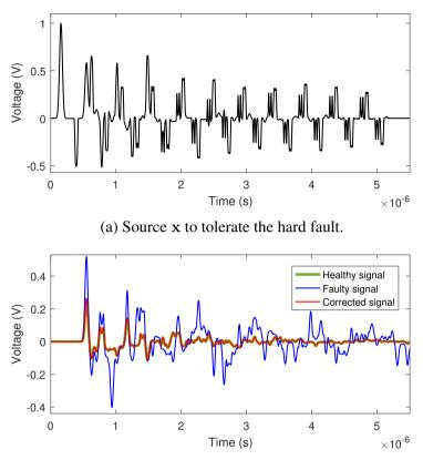
(b) Healthy, faulty and corrected voltage signals recorded by R.
