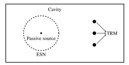
Figure 1.6: *Time-Reversal Electromagnetic Chamber: extra antennas are placed around the passive source based on the equivalence principle.*
