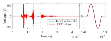
(d) Voltage signal  $\mathbf{y}'$  recorded by R' after injecting  $\mathbf{x}$  and  $\mathbf{x}'$  simultaneously.
