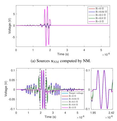
(b) Voltage signals y recorded after separately injecting the sources  $\mathbf{x}_{\rm NM}$  at different attenuation levels.
