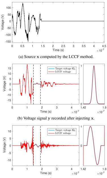
(c) Voltage signal  $\mathbf{y}'$  recorded after injecting  $\mathbf{x}$ .
