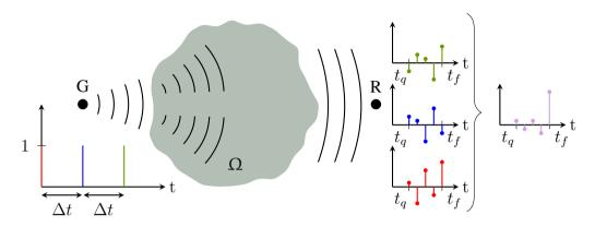
Figure 2.1: LCCF concept: the desired field is a linear combination of the impulse responses obtained over the target time  $[t_q, t_f]$ .
