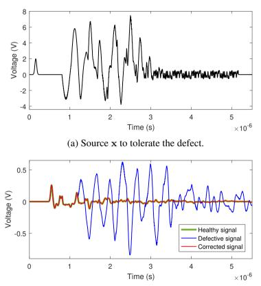
(b) Healthy, defective and corrected voltage signals recorded by R.
