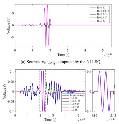
(b) Voltage signals y recorded after separately injecting the sources  ${\bf x}_{\rm NLLSQ}$  at different attenuation levels.
