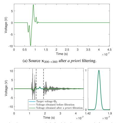
(b) Voltage signal  $\mathbf{y}_{200\to 360}$  recorded after injecting  $\mathbf{x}_{200\to 360}$  before and after *a priori* filtering.
