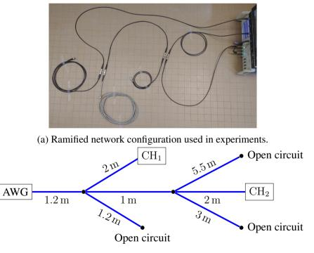
(b) Schematic diagram of the network.
