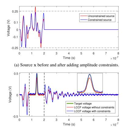
(b) Voltage signals y and  $y_{CSTR}$  recorded after injecting x and  $x_{CSTR}$ , respectively.
