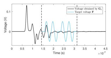
(a) Voltage signal  $y_{init}$  recorded after injecting the initial pulse  $G_1$ .
