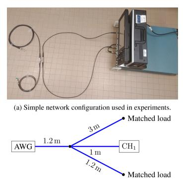
(b) Schematic diagram of the network.
