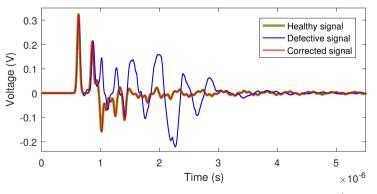
(c) Healthy, faulty and corrected voltage signals at the R'-level.
