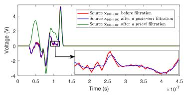
(a) Source  $\mathbf{x}_{100\to400}$  before filtering, and after *a posteriori* and *a priori* filtering. The small figure shows the effect of *a posteriori* filtering on  $\mathbf{x}_{100\to400}$ .
