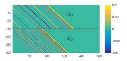
Figure 3.3: Image of the LCCF characterization matrix A (1 generator and 2 receivers).
