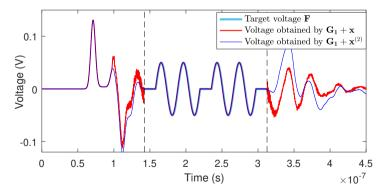
(c) Voltage signals recorded after injecting  $\mathbf{G}_1 + \mathbf{x}_{160 \rightarrow f}$  before and after filtering.
