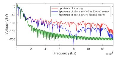
Figure 2.19: Spectra of the signal  $x_{100\rightarrow 400}$  before filtering, and after a posteriori and a priori filtering.
