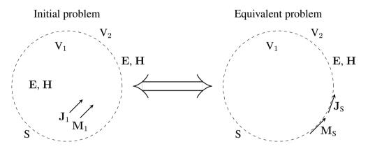
Figure 1.1: Equivalence principle concept: the source inside the enclosed volume  $V_1$  radiates to produce the electric  $\mathbf{E}$  and magnetic  $\mathbf{H}$  fields. This problem is replaced by an equivalent one; we identify sources on the enclosure of  $V_1$  that produce the same  $\mathbf{E}$  and  $\mathbf{H}$  in  $V_2$  after their radiation.
