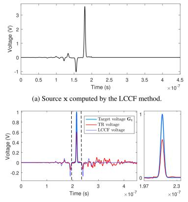
(b) Voltage signals y recorded after injecting by the LCCF source x and the TR back-propagated signals.
