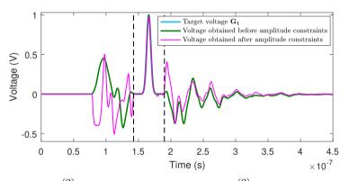
(b) Voltage signal  $\mathbf{y}_{100\to 400}^{(2)}$  recorded after injecting  $\mathbf{x}_{100\to 400}^{(2)}$  before and after adding amplitude constraints.
