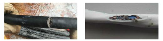
Figure 1.7: *Hard (left image [source]) and soft (right image [source]) faults appearing in wiring networks.*
