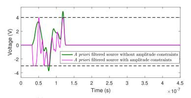
(a) Source  $\mathbf{x}_{100 \rightarrow 400}^{(2)}$  before and after adding amplitude constraints.
