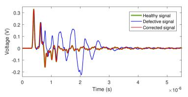
(b) Healthy, faulty and corrected voltage signals at the R-level.
