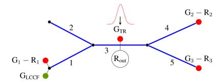
Figure 2.9: Placement of the generators and receivers for the TR and the LCCF processes.
