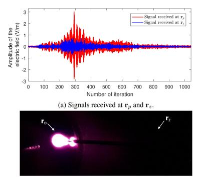
(b) Plasma is activated at  $\mathbf{r}_p$  without parasitic discharges appearing at  $\mathbf{r}_z$ .
