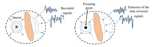
Figure 1.5: *Time-reversal principle: the source radiates through an inhomogeneous medium before ending to an array of probes surrounding the source. The divergent waves are recorded, time-reversed, and synchronously re-emitted to refocus on the source point.*
