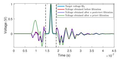
(b) Voltage signal  $y_{100\to400}$  recorded after injecting  $x_{100\to400}$  before and after filtering.
