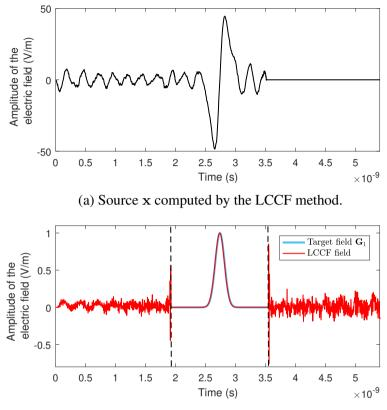
(b) Electric signal y recorded after injecting x.
