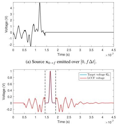
(b) Voltage signal y recorded after injecting  $\mathbf{x}_{0 \to f}$ .
