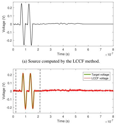
(b) Voltage signal y recorded at  $CH_1$  after injecting x.
