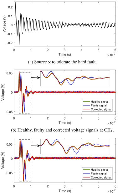
(c) Healthy, faulty and corrected voltage signals at  $CH_2$ .
