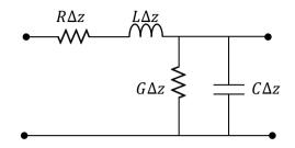
Figure 1.10: Schematic representation of the elementary component of a transmission line.
