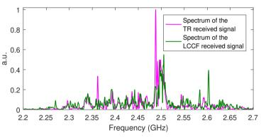
(b) Spectra of the received signals at the used bandwidth.
