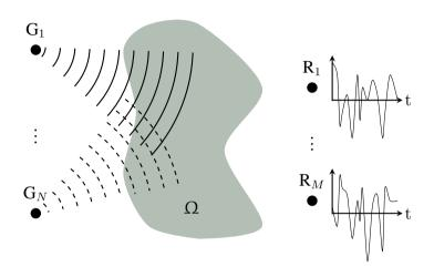
Figure 3.1: Schematic setup of the LCCF method: the source generators emit signals that propagate and interfere through a linear medium, and perhaps being distorted by inhomogeneities in the medium. Each receiver records the signal it detects.
