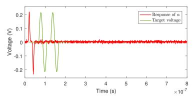
Figure 5.4: Response of  $\alpha$  used instead of the impulse response to characterize the network of Figure 5.3 at CH1.
