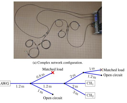
(b) Schematic diagram of the network.
