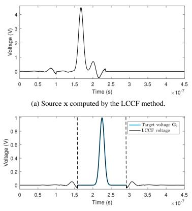
(b) Voltage signal y recorded after injecting x.
