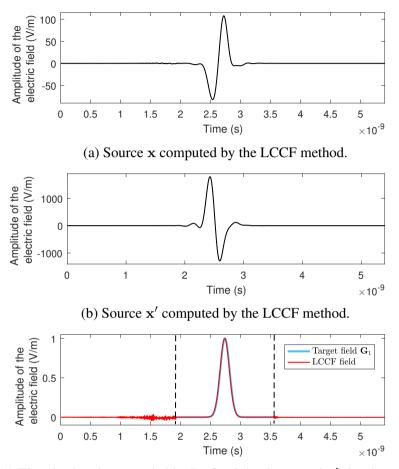
(c) Electric signal y recorded by R after injecting x and x' simultaneously.
