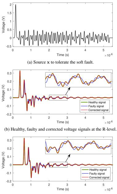
(c) Healthy, faulty and corrected voltage signals at the R'-level.
