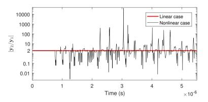
Figure 4.3: Amplitude ratios of  $|\mathbf{y}_2/\mathbf{y}_1|$  to show the nonlinearity of the system.
