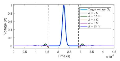
(b) Voltage signals y recorded after separately injecting the sources x at different attenuation levels.
