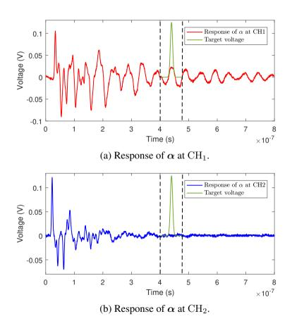
Figure 5.10: Response of  $\alpha$  used instead of the impulse response to characterize the network of Figure 5.9 at CH1 and CH2.
