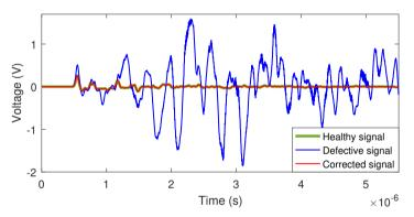
(b) Healthy, defective and corrected voltage signals recorded by R.
