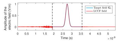
(d) Electric signal  $\mathbf{y}'$  recorded by R' after injecting  $\mathbf{x}$  and  $\mathbf{x}'$  simultaneously.
