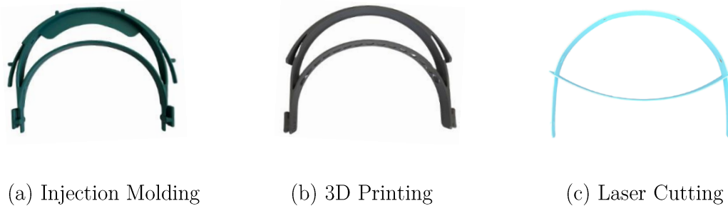
Figure 6.2 Faceshield brackets, Manufactured by Sigma Clermont
