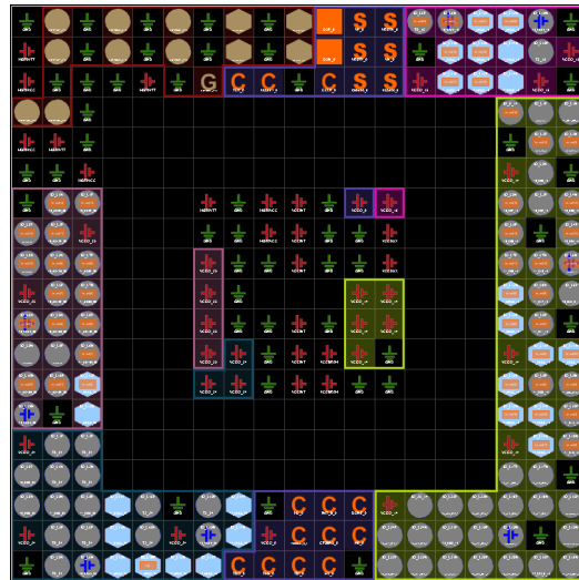
FIGURE B.4: I/O planning of NPS1 RTL model. NPS1 has one 1-bit input port clock and two 24-bit output ports rw and rw , so totally 49 pins are distributed to these three ports.
