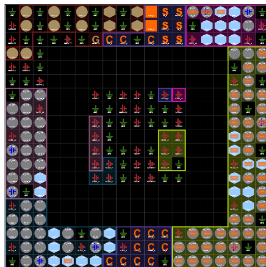
FIGURE B.6: I/O planning of ENPS1. 49 pins are used to represent I/O ports.
