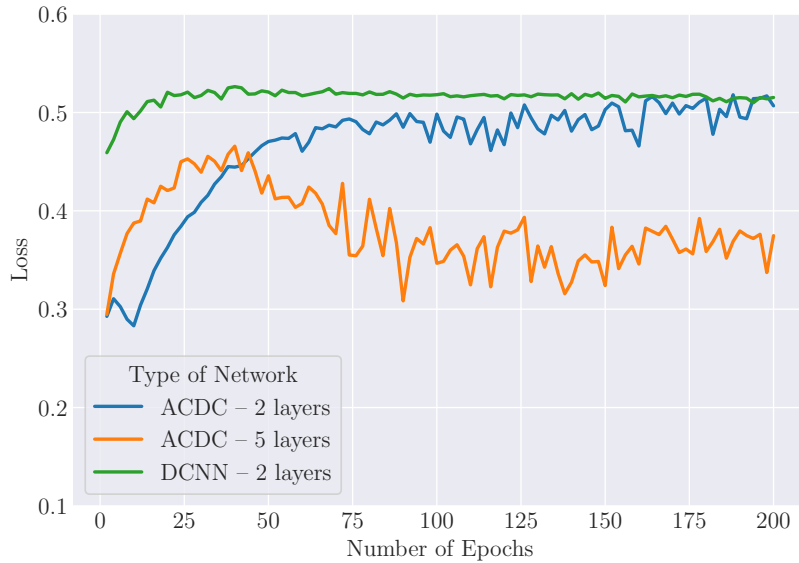
Figure 4.4: Comparison of the training loss of DCNNs and ACDC networks on a CIFAR-10 dataset.
