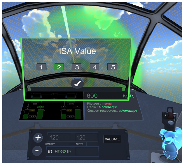
Figure 12: Example of self-reporting method in an IVE. Instantaneous Self-Assessment (ISA, measure of the user's MW using 5 different ratings [287]) in a VR Flight Simulator [172].
