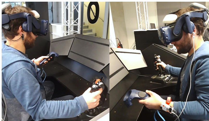
Figure 54: Multiple views of the experimental setup. The user is wearing a Vive Pro Eye equipped with sensors on the headset, a Shimmer3 GSR+ on his left hand, and using a joystick and a Vive Controller on the cockpit.
