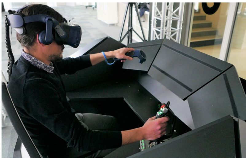
Figure 42: Picture of the experimental set-up. The user is wearing a Vive Pro, and using a joystick and a Vive controller on the cockpit.
