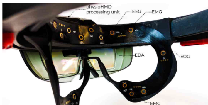
Figure 20: PhysioHMD [27]. Example of a module which integrates physiological sensors directly on the headset.
