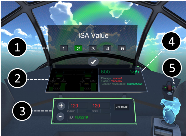
Figure 38: Virtual cockpit view. (1) Instantaneous Self Assessment (ISA) interface. (2) Resources management task interface (deactivated); when activated, the interface lit up (with a green outline). (3) Communication task interface (activated); when deactivated, the interface lit off (no green outline). (4) Informative panel which gives information about which task is activated or not at the current time. (5) Virtual representation of the joystick used to pilot the aircraft and of the right hand. The left hand is represented in the same way, but tracked by a Vive Controller and animated depending on the interaction.
