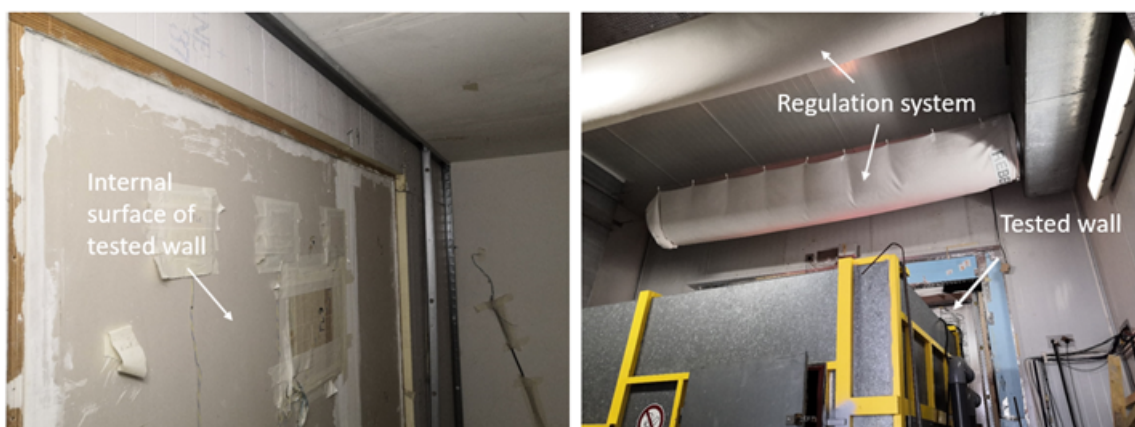
Figure 5.12: (left) Interior and (right) exterior views of the climatic chamber at LNE.
