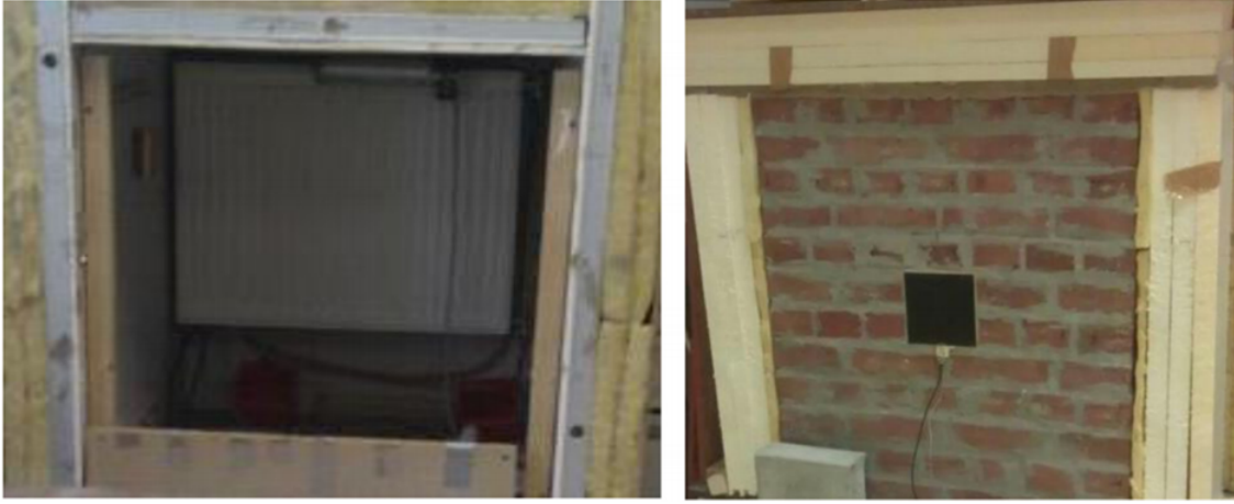
Figure 1.15: The real view of (left) the heating box and of (right) the experimental setup on the front face of the wall in [33].
