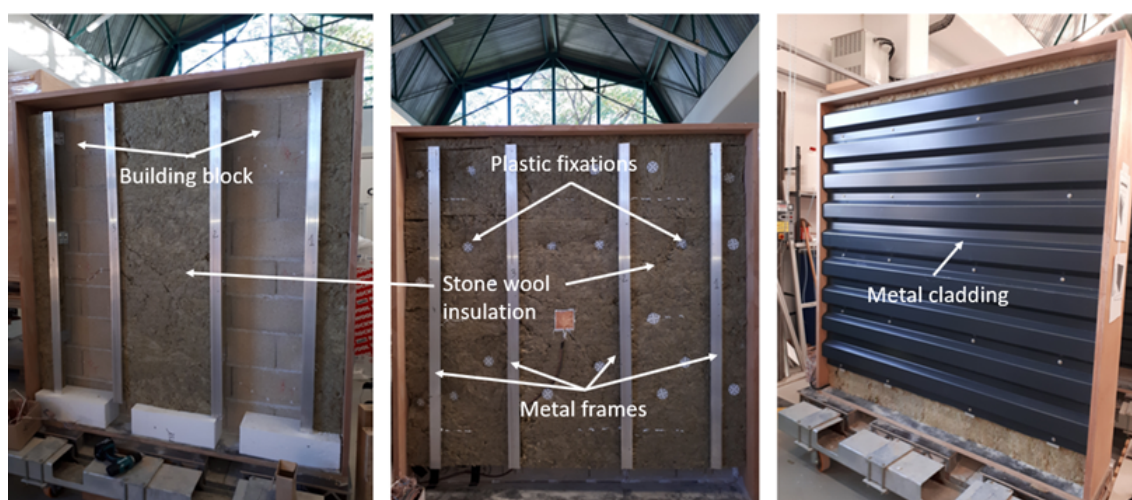
Figure 5.4: Tested EWI wall: (left) Real view of building block layer and metal frame, (middle) of the wall without BA13 from interior view and (right) of the metal cladding of the complete wall.
