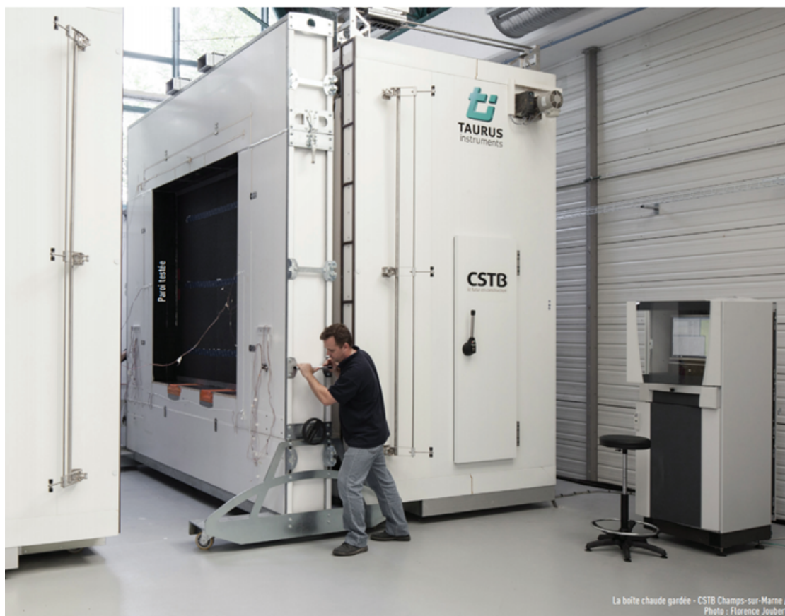
Figure 5.8: Guarded Hot Box device at CSTB [87].
