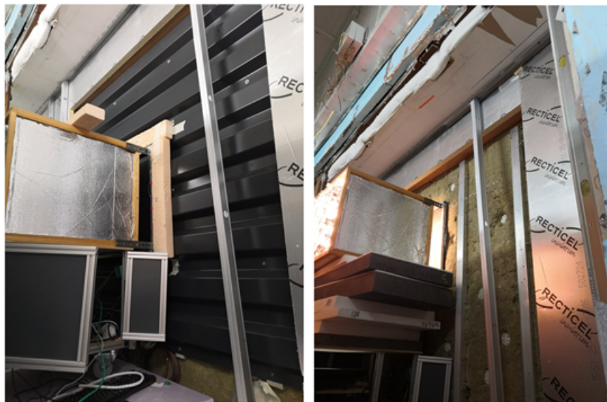
Figure 5.18: Prototype setup on (left) the metal cladding and (right) the external surface of insulation layer of the EWI wall.
