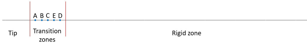
Figure 3.41: Modeling of the rigid guidewire whose elastic mechanical properties vary according to different transition zones ( Menut, 2017 )
