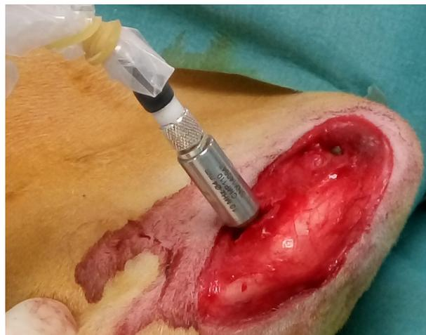
**Figure 8.3** – Measurement configuration of the ultrasonic indicator using the ultrasonic transducer screwed into a dental implant.
