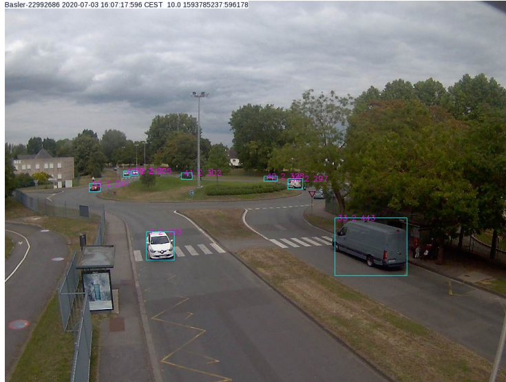
Figure 5.10: Bounding boxes of detected vehicles from the image acquired by the intelligent infrastructure. Université Gustave Eiffel results.
