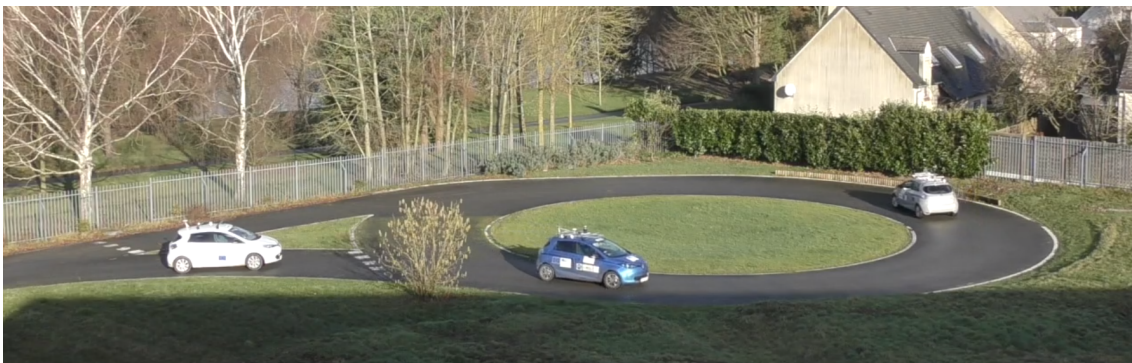
Figure 3.18: The experimental circuit “Seville” and the experimental Renault Zoés used during the real outdoor tests. In our configuration, the white car (fully autonomous) is the AD vehicle, while the others are the road users (manually driven).
