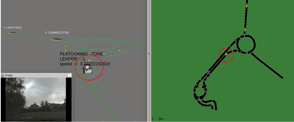
Figure 2.6: Hybrid simulation experiment on the circuit Seville. On the right of the figure, the MD traffic generation in SUMO (yellow cars) and the AD vehicle (gray car, in the red circle). On the left, the corresponding intelligent vehicle framework with the same obstacles (yellow rectangles). As all the MD vehicles are simulated, they do not appear in the AD vehicle context camera
