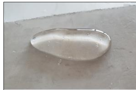
Figure 96 : Waterproofing of C65P30H5DM
