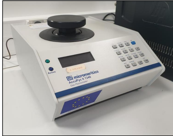
Figure 29 : Absolute density measuring device.
