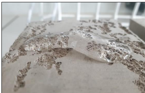
Figure 95 : Waterproofing of C55P30H15PM
