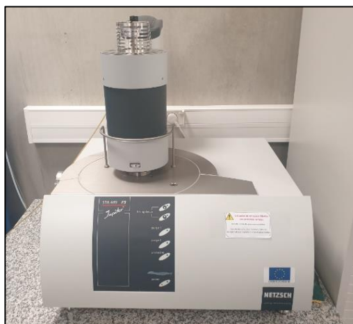
Figure 37 : Thermogravimetric analyses (TGA) device
