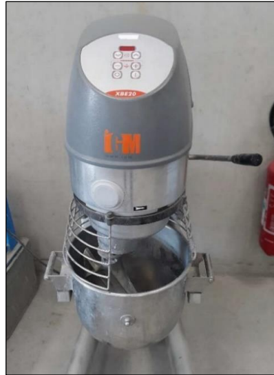
Figure 27 : IGM mixer used to produce mineral suspensions.
