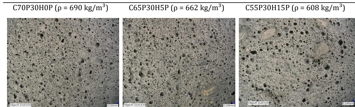
Figure 61 : Pore structure evolution with increasing amount of hemp shiv using the preformed method.
