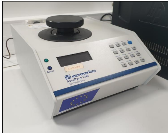
Figure 29 : Absolute density measuring device.
