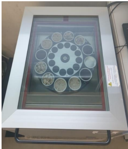
Figure 39 : Device used for DVS testing (ProUmid)
