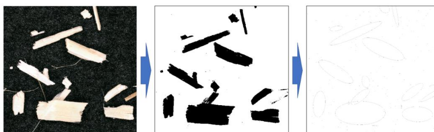
Figure 24 : Protocol of granulometric analysis by image treatment (Scan, conversion of the gray scale and adjustment in the form of ellipses).
