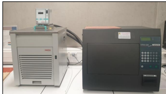
Figure 34 : Thermal conductivity test device.
