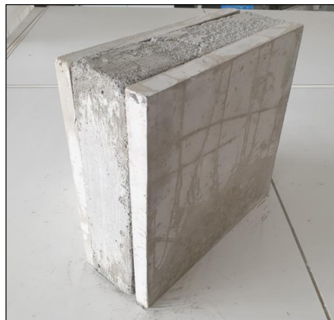
Figure 103 : Sandwiched concrete BBISE.
