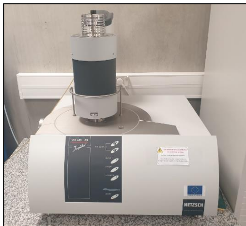
Figure 37 : Thermogravimetric analyses (TGA) device
