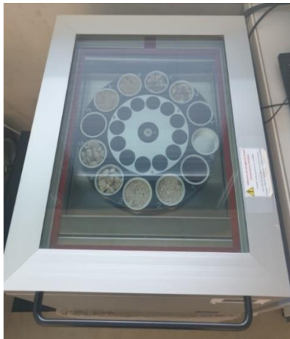
Figure 39 : Device used for DVS testing (ProUmid)
