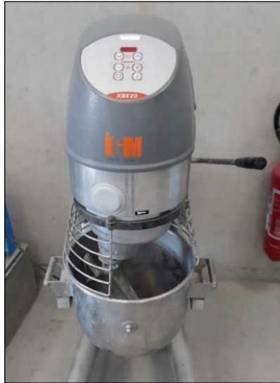
Figure 27 : IGM mixer used to produce mineral suspensions.
