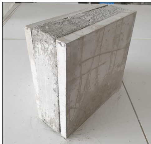
Figure 103 : Sandwiched concrete BBISE.
