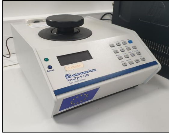
Figure 29 : Absolute density measuring device.
