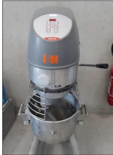
Figure 27 : IGM mixer used to produce mineral suspensions.
