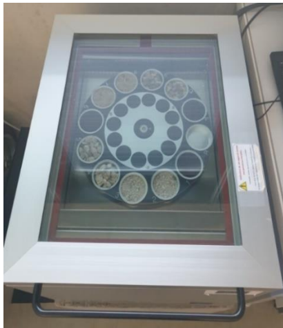
Figure 39 : Device used for DVS testing (ProUmid)
