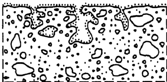
Figure 88 : Schematic representation of mass water repellents on the pores [203].
