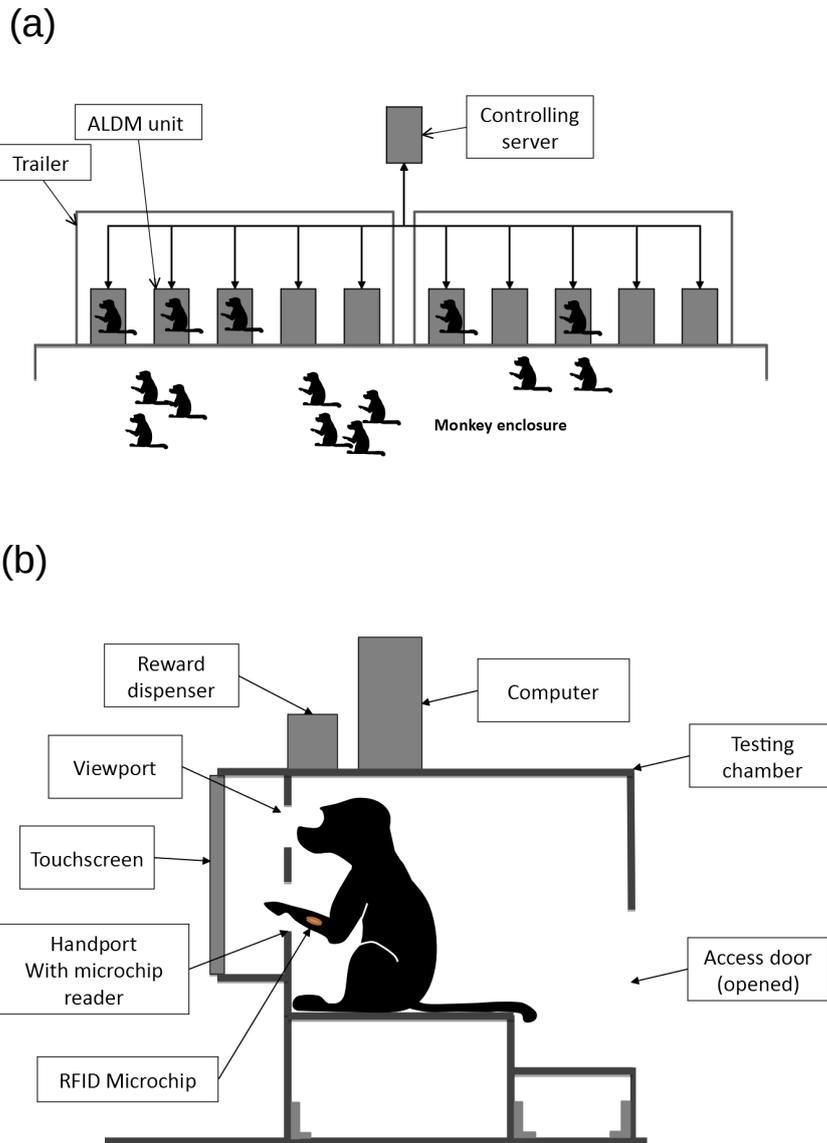
FIGURE 2.4. : **ALDM self-testing system.**(a) Schematic of the ALDM system's organization. (b) Details of the ALDM testing unit
