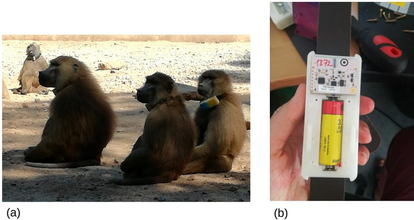
FIGURE 2.2. : (a) : Individuals in the enclosure, wearing collars with the attached boxes embedding the tags. (b) : Interior of a single box containing the tag (top) and the connected battery (bottom)
