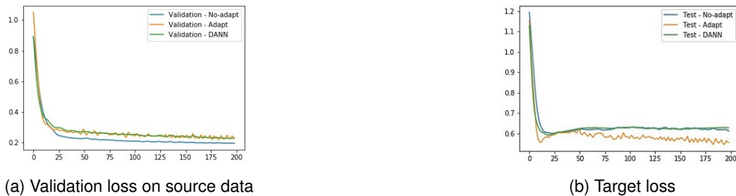
Figure 4.6: Training curves for Single Source DA: without adaptation, the target loss increases as the validation loss keeps decreasing. DANN exposes the same behaviour as the target loss of AHDM decreases.
