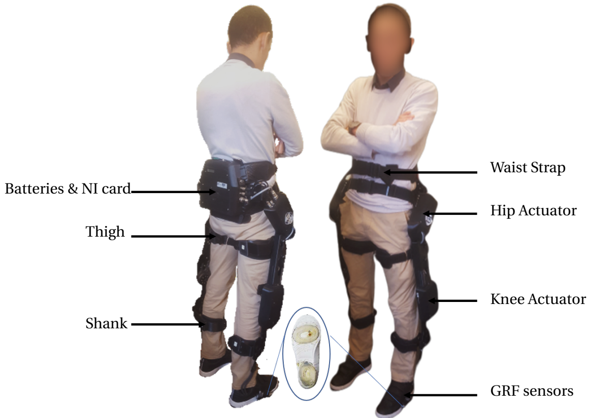
Figure 3.7: A subject wearing the ANGELEGS Exoskeleton
