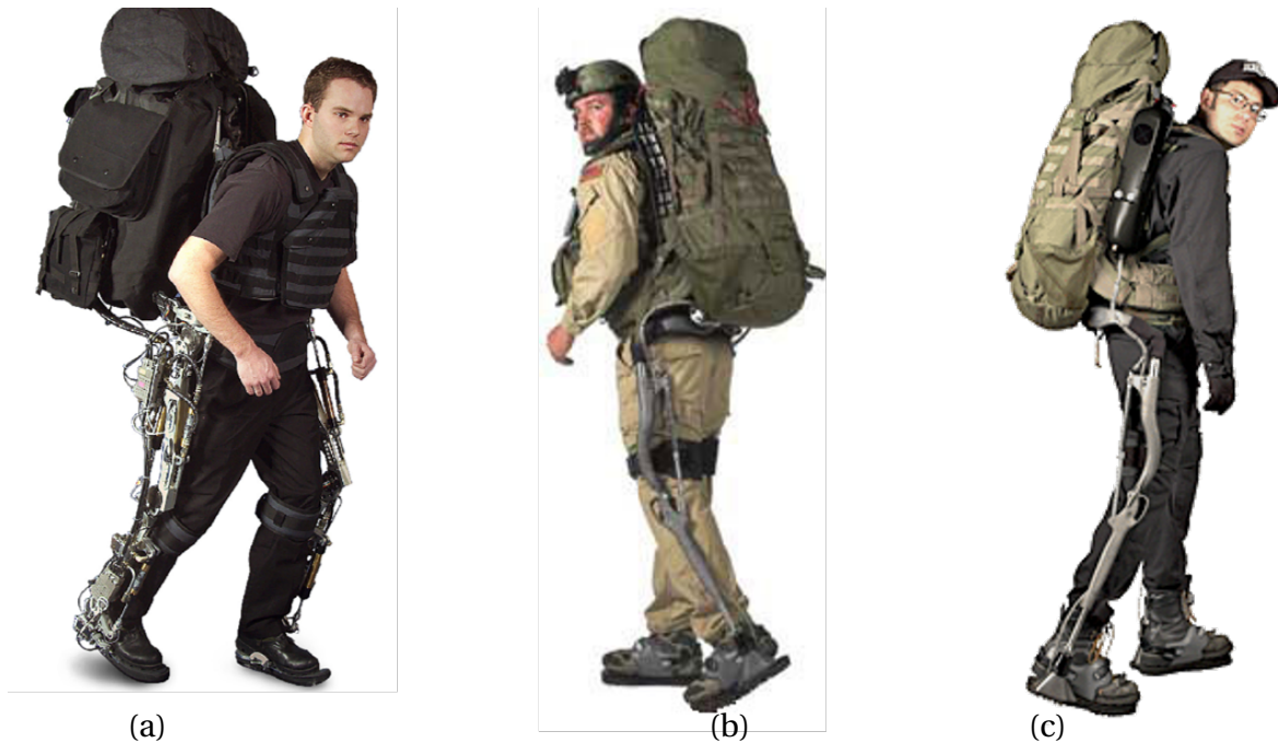
Figure 2.1: (a) BLEEX, (b) ExoHicker, (c) ExoClimber.
