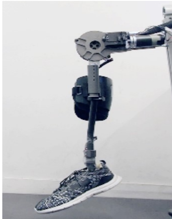
Figure 3.12: Identification of the SEA-actuated knee joint dynamic model
