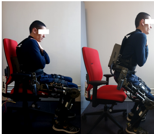
Figure 7.13: Pre-extension and extension phases of STS movement.
