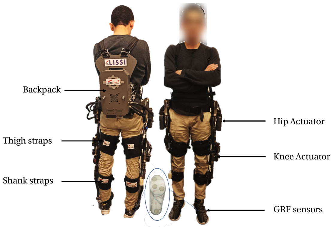
Figure 3.6: A subject wearing the EROWA exoskeleton
