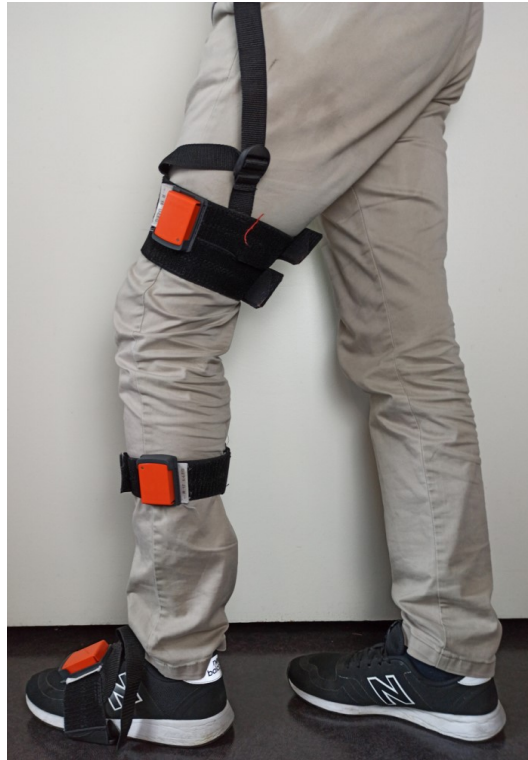
Figure 3.1: Xsens wireless MTW IMUs attached at thigh, shank and foot.
