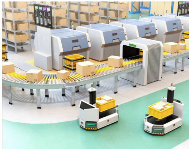
FIGURE 1.3 – Un atelier de type FMS.
