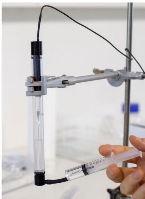
Figure 2: Sulfide sensor with the calibration cap mounted. Calibration solution is injected with the 10 ml syringe.
