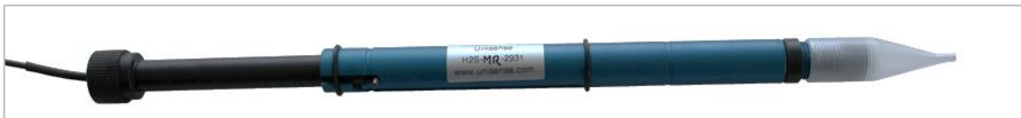
Figure 3: H 2 S sensor in the Microrespiration guide.
